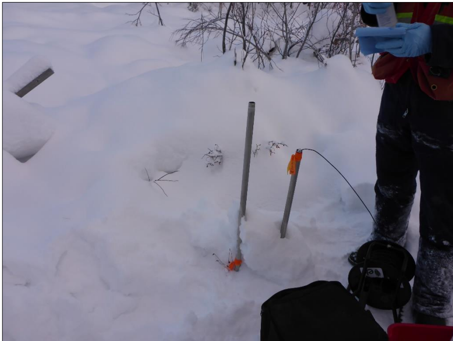
Photo 2: View of drive point wells GSI-DC-02A and GSI-DC-02B. Photo taken on January 30, 2017.
