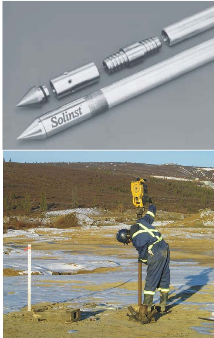
Figure 2-1: Drive-point Profiler (above) and Pionjar Hammer (below).
