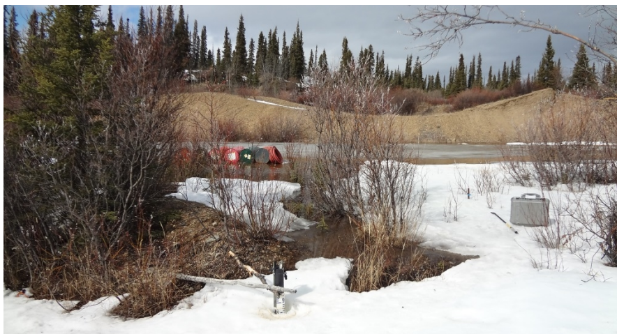
Photo 16: H-VC-R stilling well, with water from parking lot flowing into creek at location.
