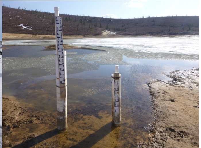
Photo 61. H-TP staff gauges (May 13, 2015).
