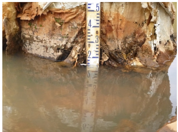
Photo 18. H-SEEP – seepage pond staff gauge.
