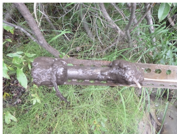
Photo 24. H-PC-DSP – showing logger with sediment in stilling well.
