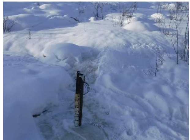
Photo 4. H-DC-M WP – looking upstream at weir pond. Stilling well frozen in ice and soil.
