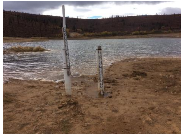
Photo 10. H-TP – overview of tailings pond showing wetted lower staff gauge.
