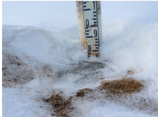
Photo 10. H-TP – tailings pond lower staff gauge encased in ice.
