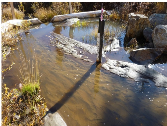
Photo 7. H-DC-M WP downstream view of weir pond filled in with sediment (Sept 16, 2014).
