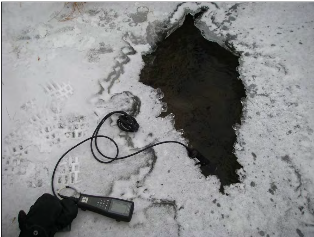
R1 – Conductivity logging for salt slug flow measurements
