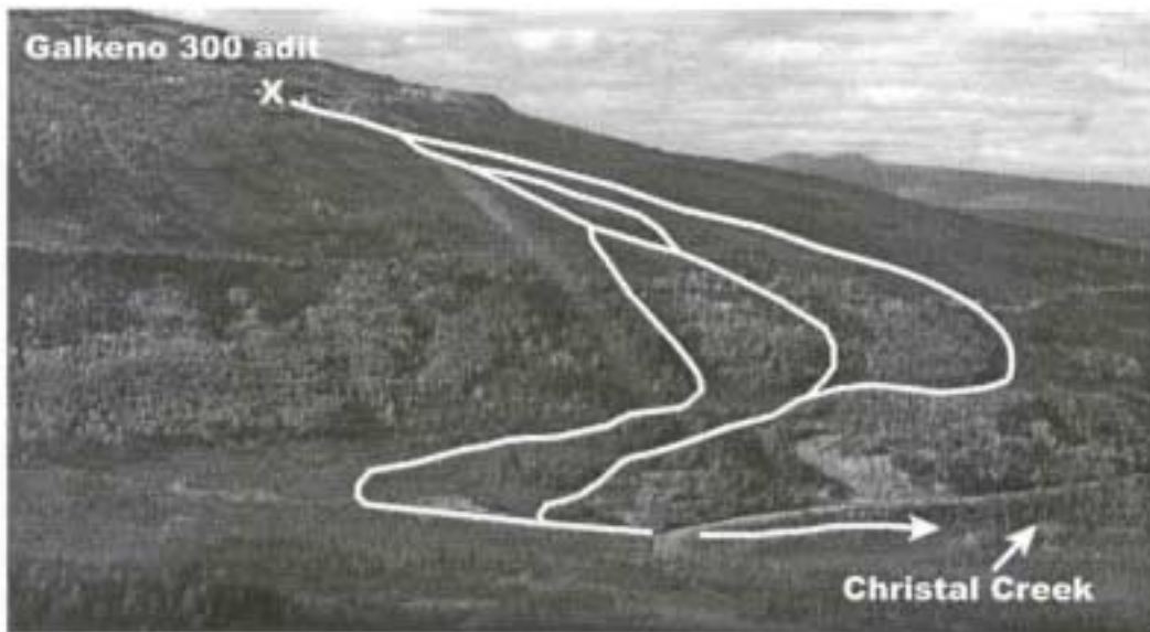
Figure 11 – Generalized pattern of surface and sub-surface flow paths from the Galkeno 300 adit to Christal Creek (adapted from MacGregor and Li 2001a).
