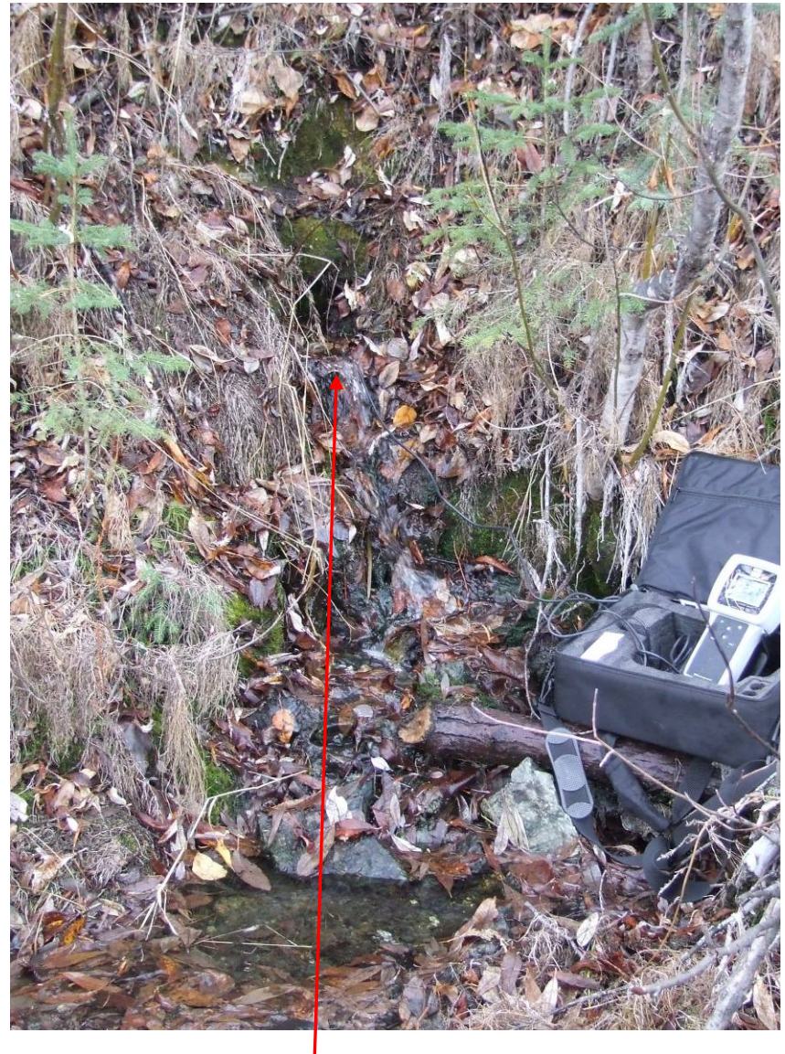
GWCC-3, groundwater seeps from the hillside at the base of the waste rock dump, October 4 th , 2012.
