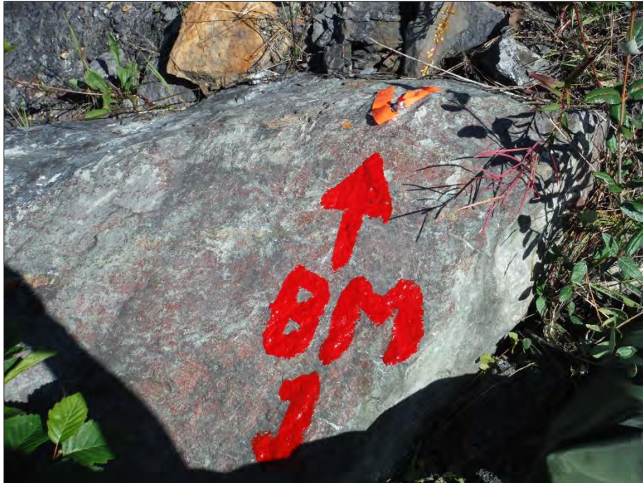
Pressure Sensor Located in Hudgeon Lake – near Site E1(H) Continued Benchmark 1. Rock bolt in boulder just above the shoreline of Hudgeon Lake
