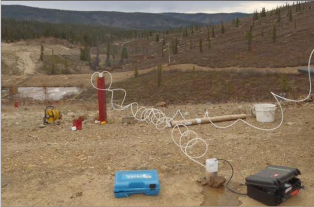
Photo 15: MW09-23 on the Tailings Dam Crest. Note the two hose bladder pump set-up and the flow through cell for monitoring field parameters. June 2, 2012
