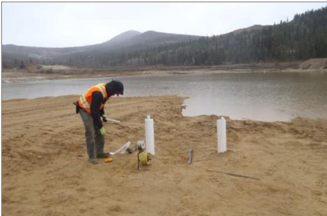
Photo 1: MW09-01 and MW09-02 in the Southeast Tailings. Also shown in this photograph are the Heron Instruments water level sounder and cable for the Solinst Levelogger used during the sampling event. June 2, 2012
