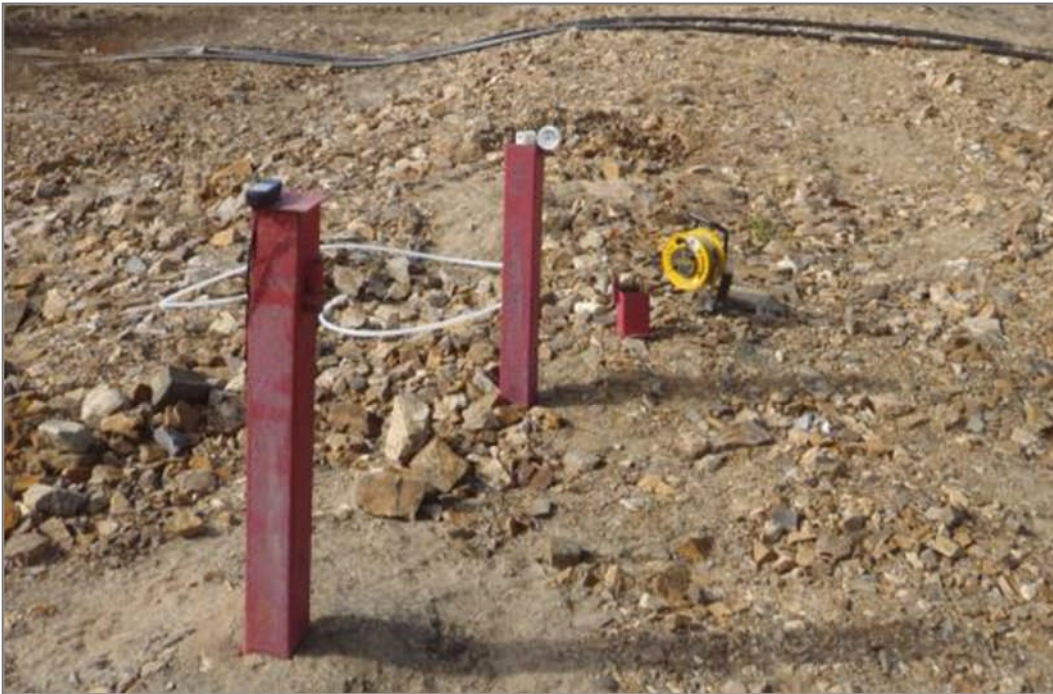
Photo 12: MW09-20, Seepage Pond Crest. Note the thermistor casing in the foreground. June 2, 2012
