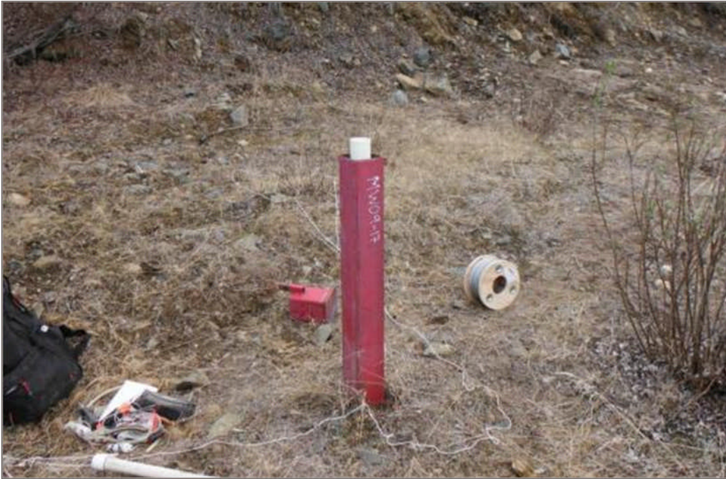
Photo 9: MW09-17, East and Downgradient of Mill Complex. June 1, 2012
