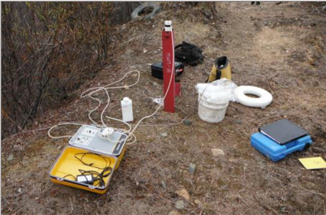
Photo 10: MW09-18, East and Downgradient of the Mill Complex. Note peristaltic pump set-up. June 1, 2012
