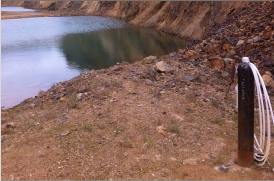
Photo 31: GLL07-03 Located in the Open Pit. Note the barologger attached to the casing lid. June 27, 2012
