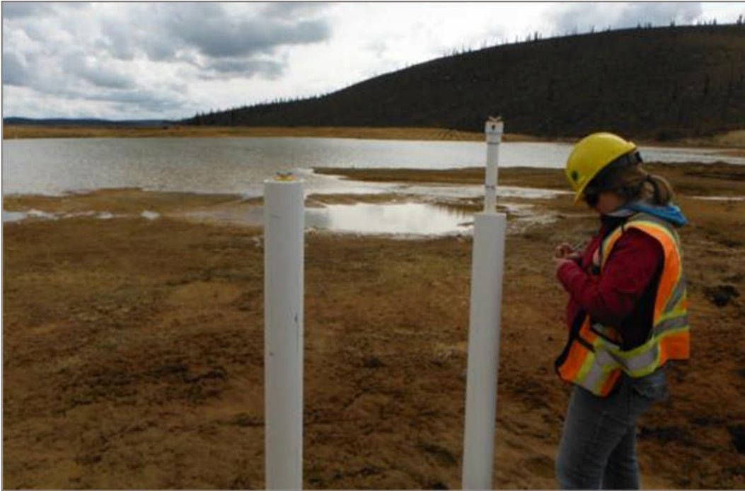
Photo 25: MP09-09 and MP09-10 Mini-Piezometers Located in the West End of the Tailings Pond. June 4, 2012
