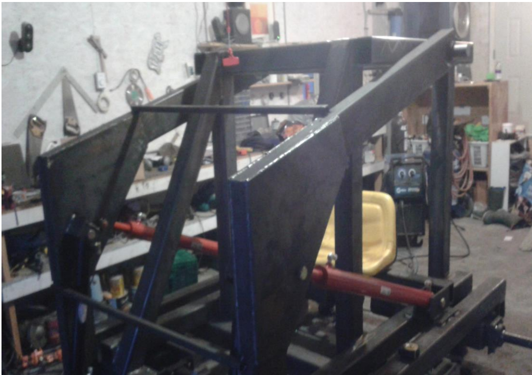
Fig. 2 Bent arms, frame, and shortened wheel base.
