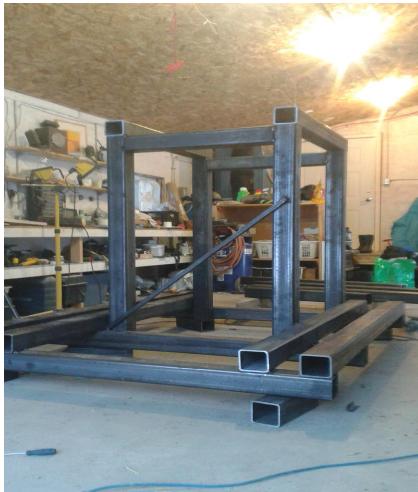
Fig 1. Frame being squared and welded.
