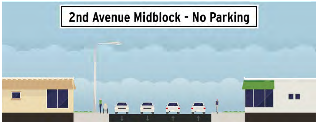
Figure 3: 2 nd Avenue Midblock no Parking Cross Section
