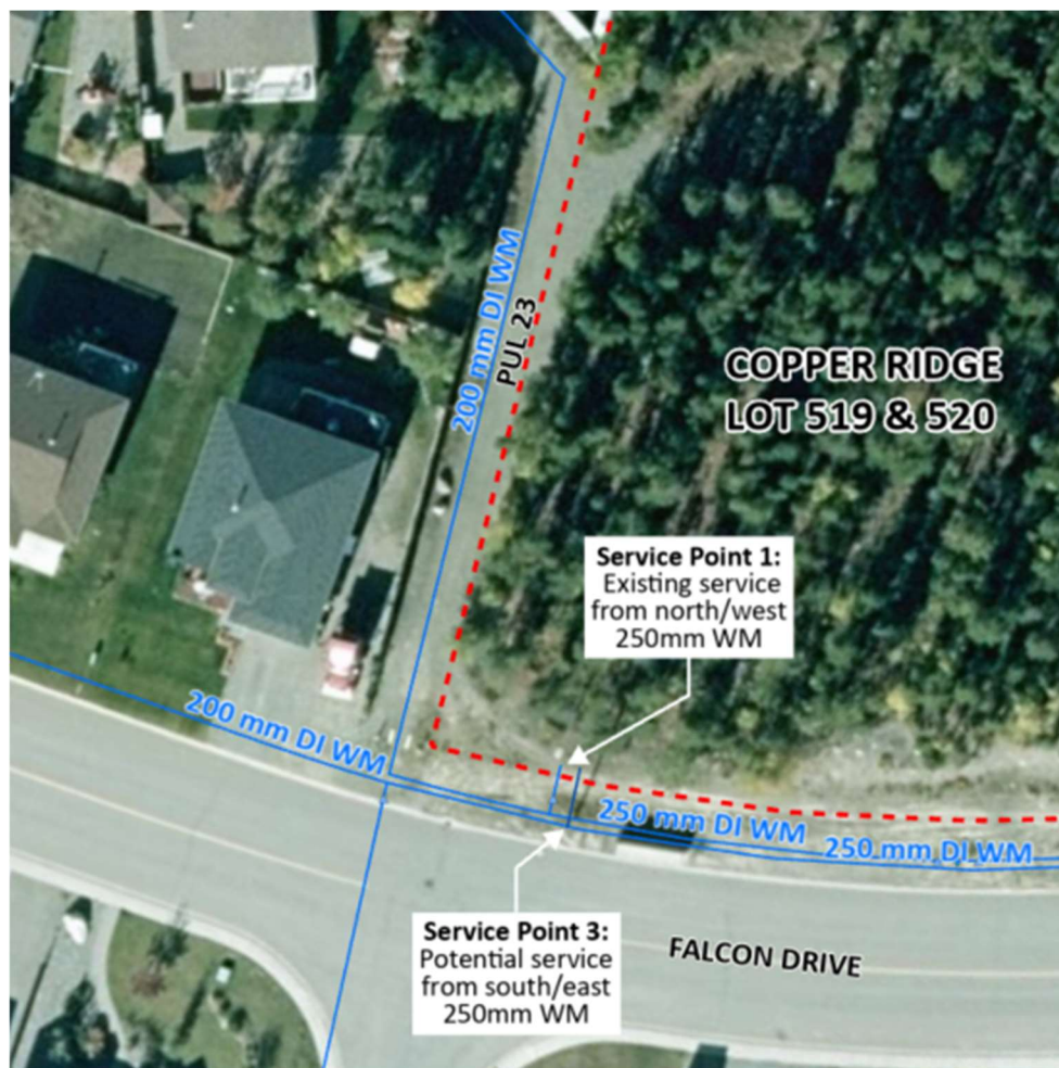
Figure 2-2A Existing watermains on Falcon Drive (between Iron Horse Drive and North Star Drive)
