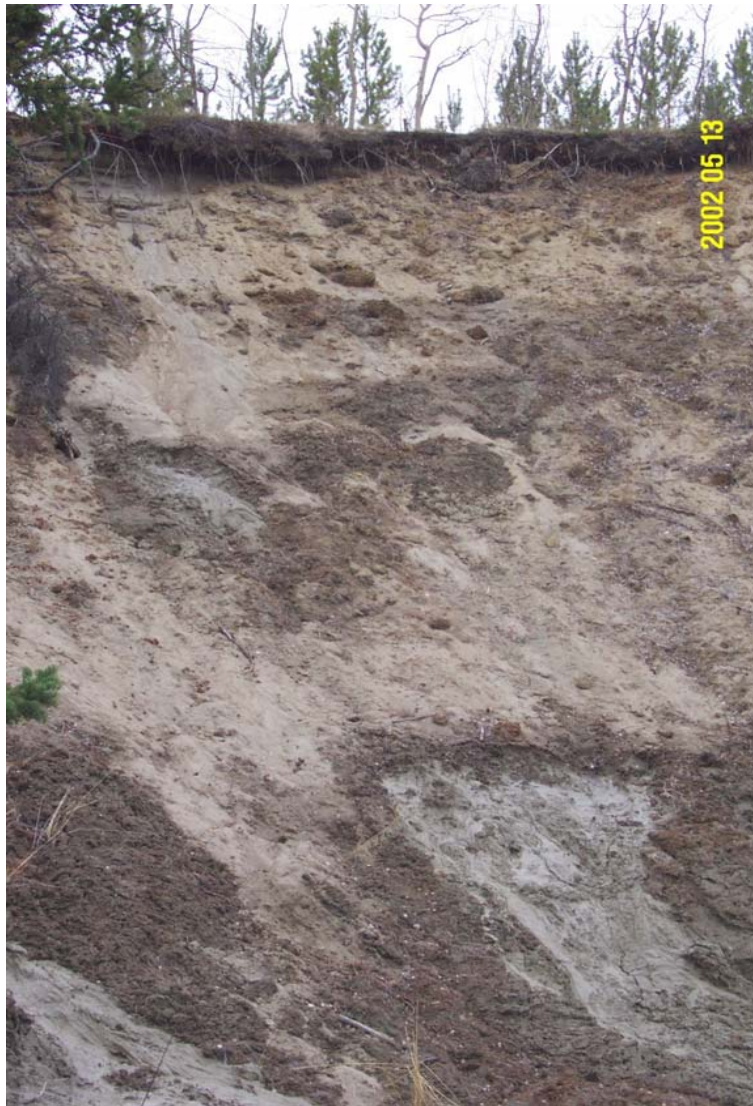
Photograph 7: May 2002. Details of thaw/flow zones within the active headscarp of the Lambert Street Slide.
