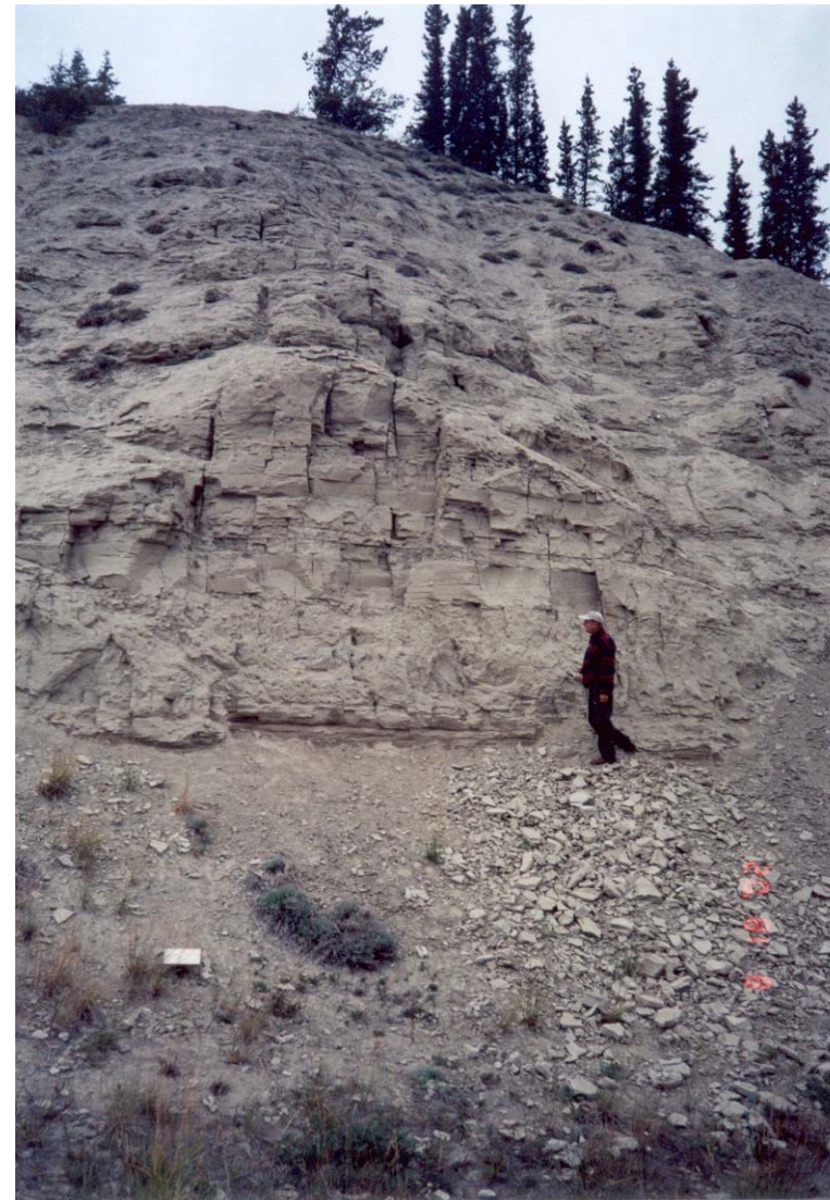
Photograph 15. August 2002. Sub-vertical silt bluffs with toppling debris at viewpoint on historic east airport road near Hawkins Street.
