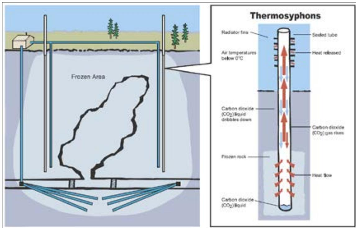
**Figure 6.** The frozen block method uses thermosyphons to ensure subsurface contaminants remain frozen through time. This system is being used for the Giant Mine remediation project near Yellowknife, NWT (INAC, 2007).
