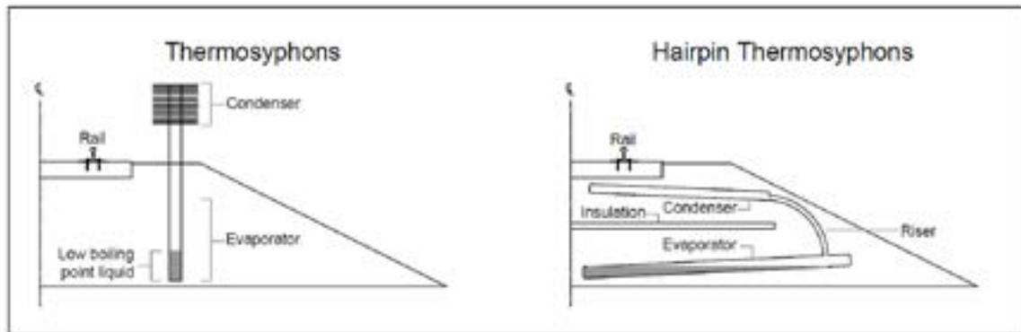
Figure 11. Thermosyphon designs (Regehr et al., 2012).
