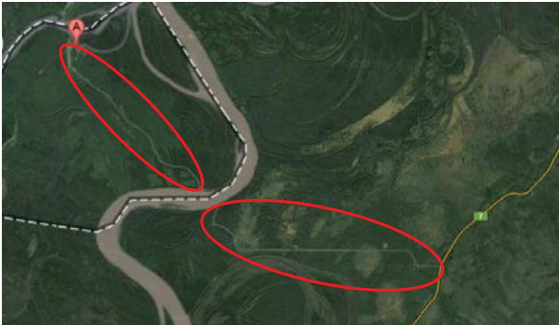
**Figure 14b.** A new 23 km, all-weather access road was opened to Nahanni Butte in 2010 and runs from Highway #7 to the east bank of the Liard River. A water taxi crosses the Liard River in the summer, and an ice road is used in winter, and then the access road continues to the community of Nahanni Butte.
