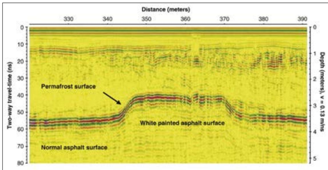
**Figure 8.** Radargram of Ground Penetrating Radar (GPR) (Jørgensen and Andreasen, 2007).
