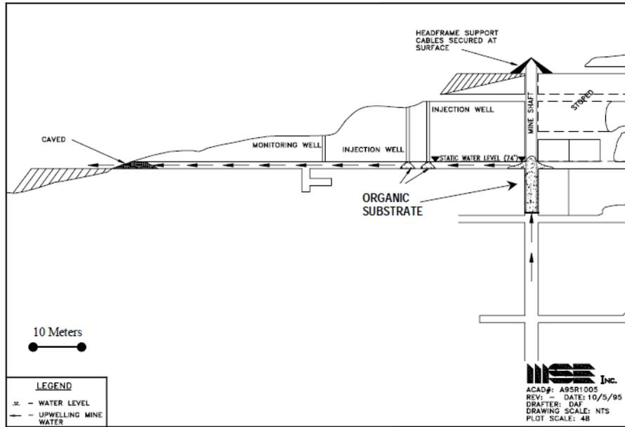
Figure 13: Underground bioreactor at Lilly/Orphan Boy Mine, Montana (Nordwick et al, 2006, p. 1412).
