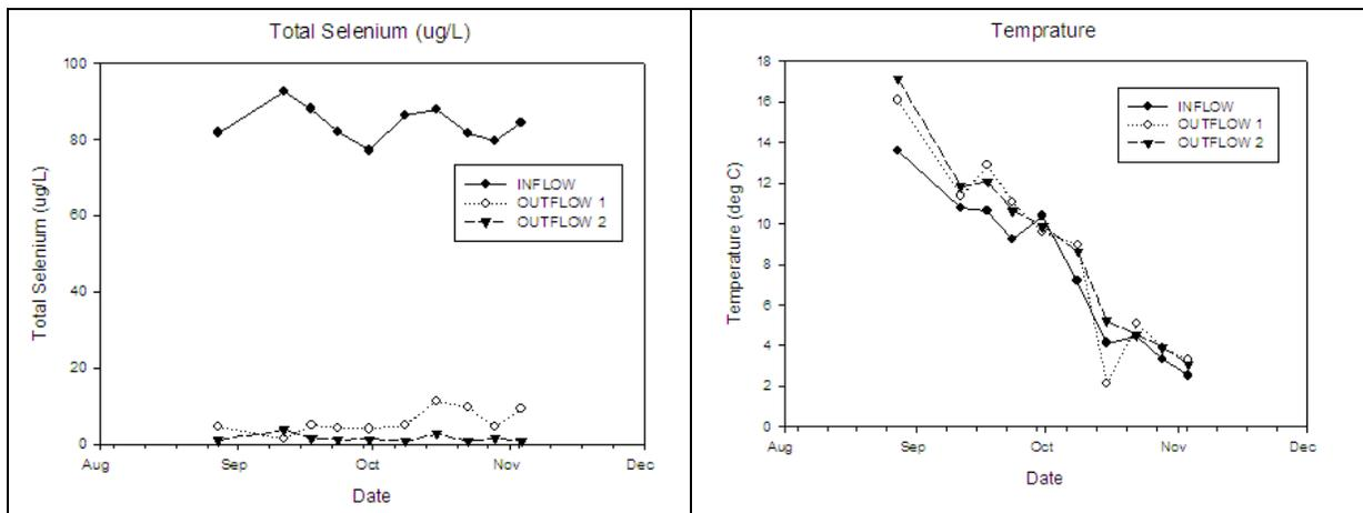
**Figure 9: Selenium removal as a function of temperature at Smoky River Coal (Sobolewski, 2010, p. 2)**
