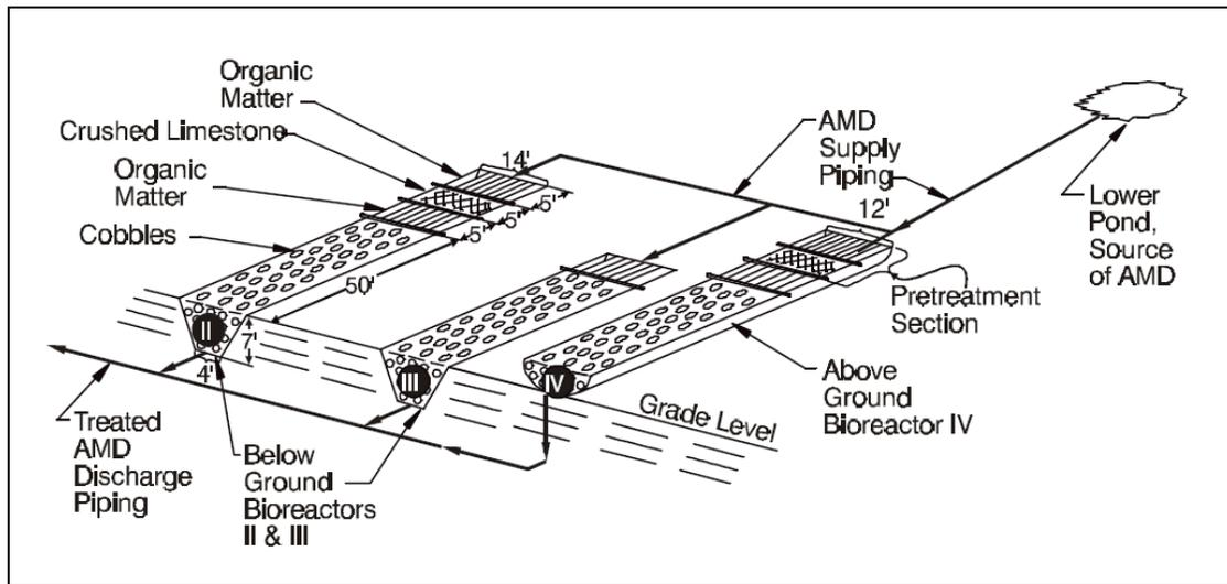
Figure 15: SRB bioreactors at Calliope Mine (Wilmoth, 2002, p.21).
