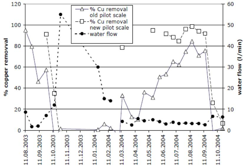
**Figure 10: Copper removal (%) by pilot anaerobic reactors versus water flows (Ettner 2007, p.3)**
