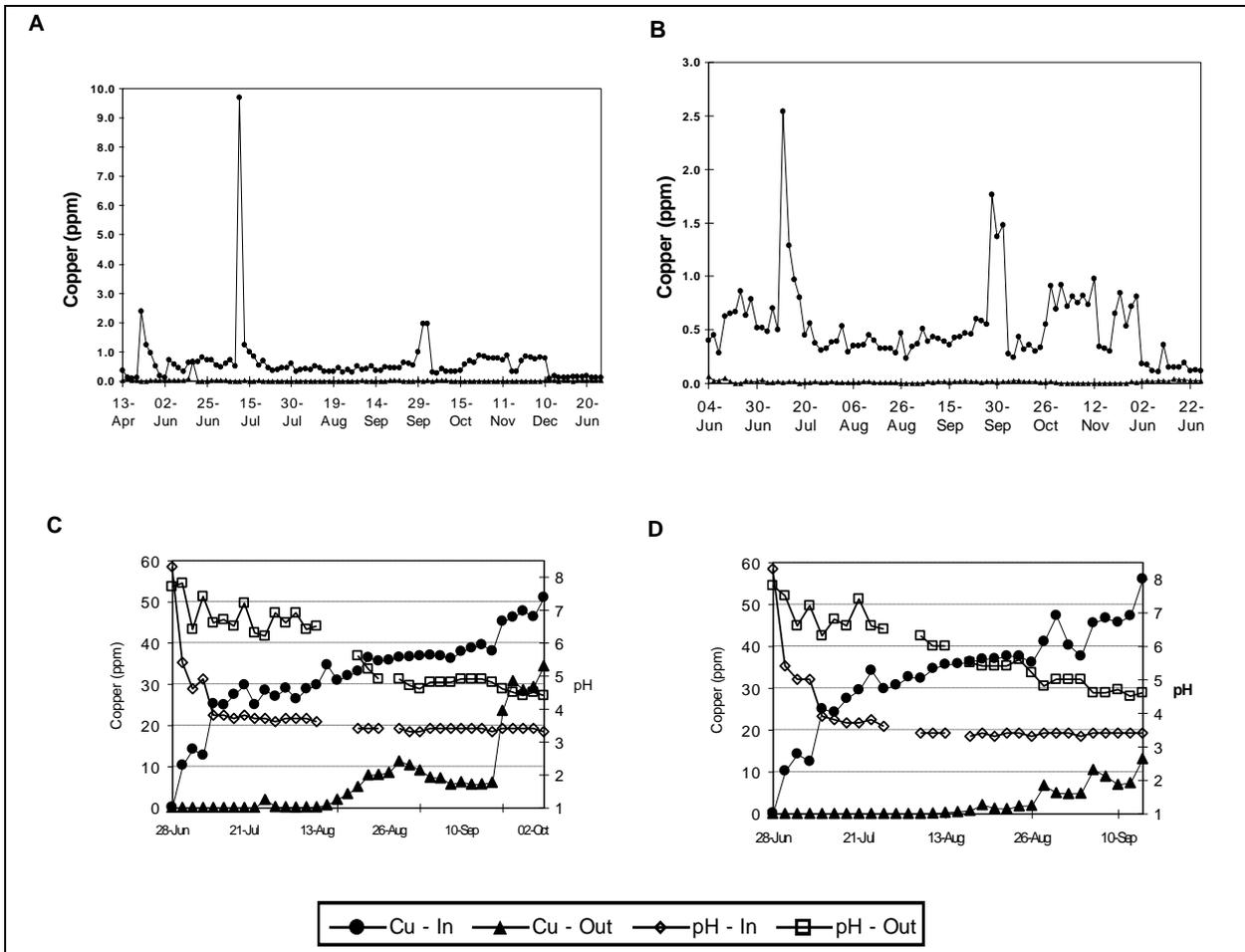
**Figure 12: Copper concentrations and pH of influent and effluent for the large (A, C) and small pond (B, D) at low strength (A, B) and high strength feed (C, D) (April 1992 to Oct 1993, Sobolewski et al, 1994, p. 686). Note different scales used in A and B.**
