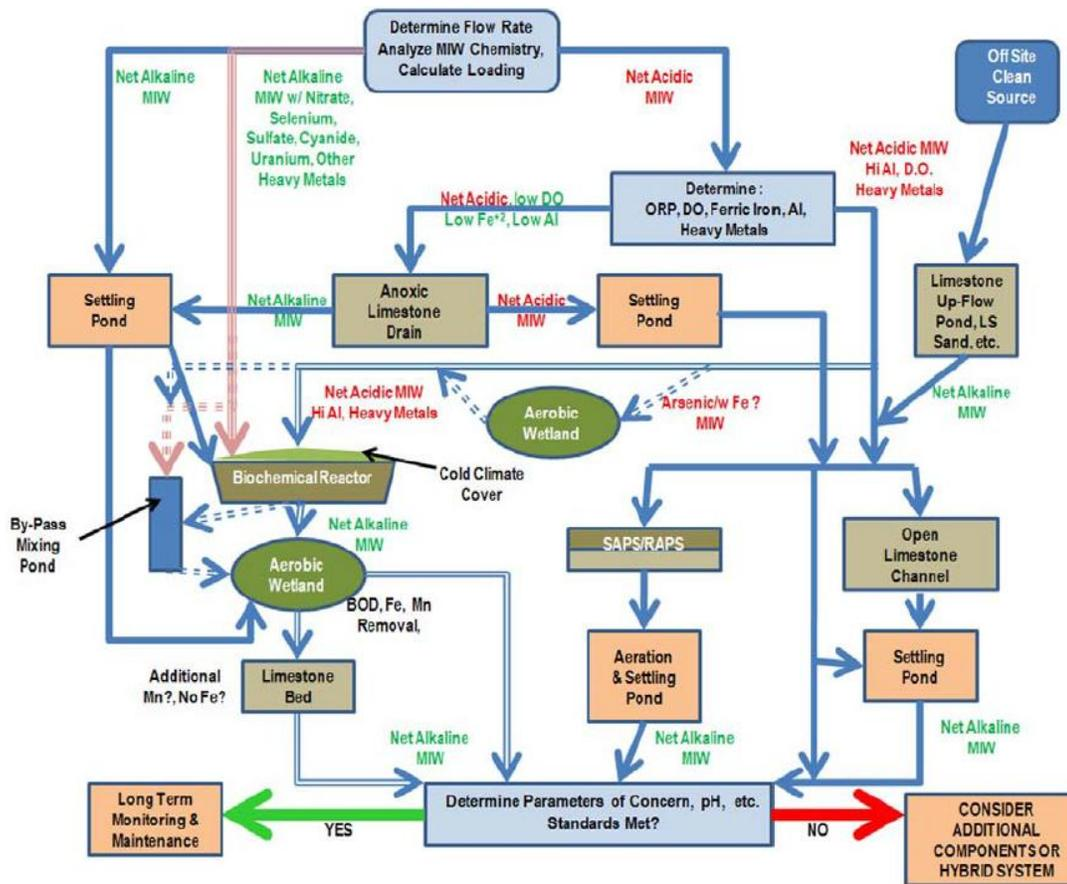
Figure 1: Flow chart for selecting PTS based on water chemistry and flow (adapted from Hedin et al, 1994 by Gusek, 2008, p. 4).
