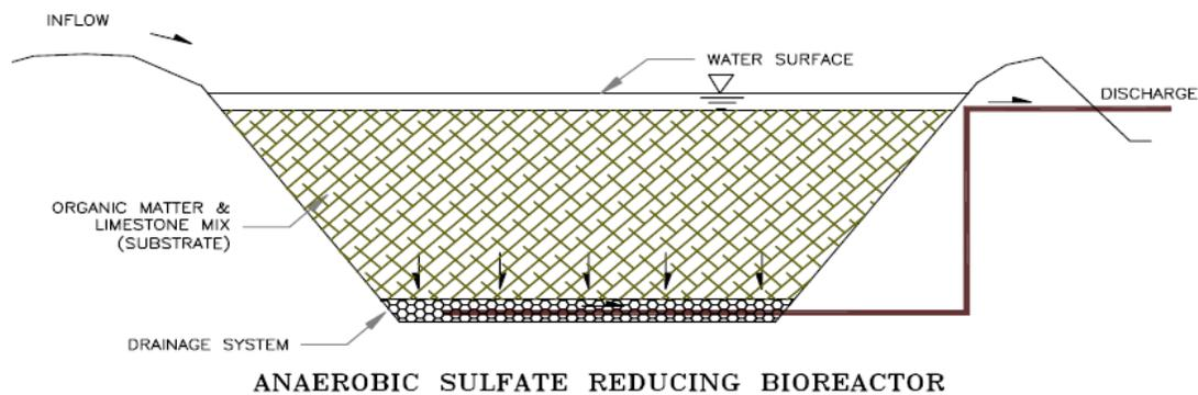
**Figure 3: Typical bioreactor design (Gusek, 2002, p. 3).**
