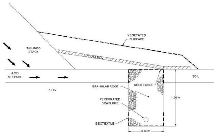
Figure 18: Cross-section of the collection ditch at the Cadillac mine PTS illustrating the use of insulation above the seepage (Kuyucak, et al, 2006, p.989).
