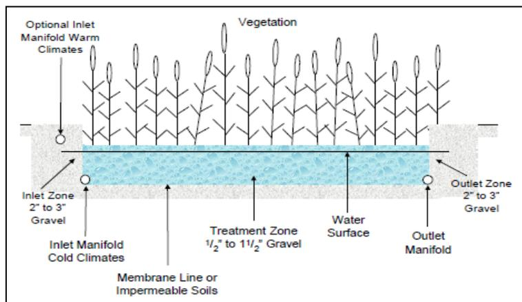
Figure 2b: Sub-surface flow wetland (adapted from a drawing by SC Reed from EPA, 2000b, p. 1).
