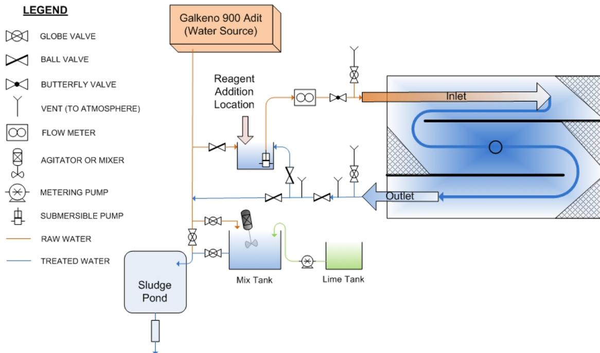
**Figure 8: Layout of Galkeno 900 bioreactor (Alexco, 2012, p.7).**
