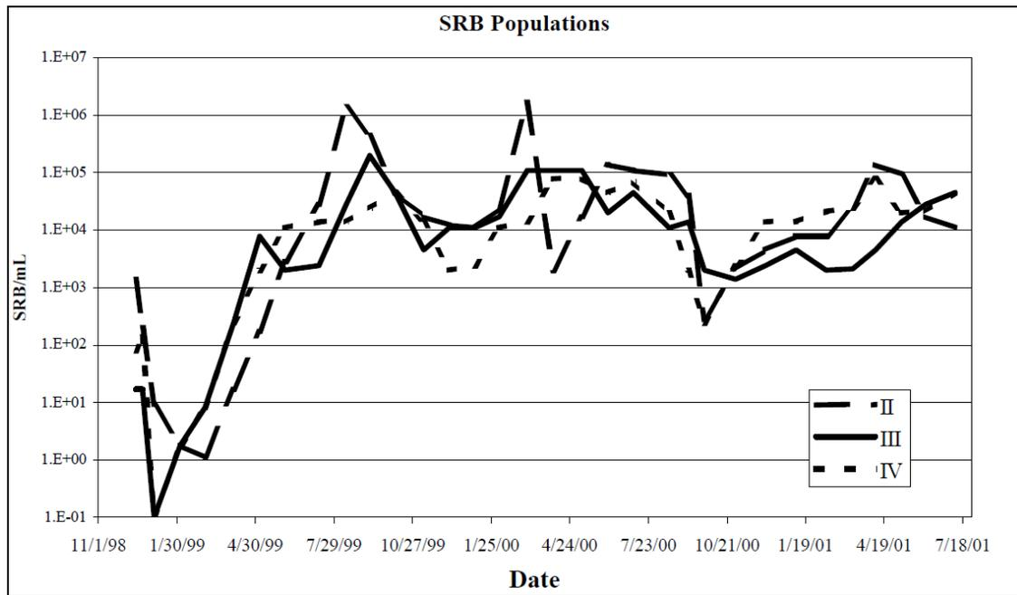
Figure 16: SRB population variation over 3 years in below-ground (II and III) and above-ground (IV) bioreactors at Calliope mine, Montana (Wilmoth, 2002, p. 35).
