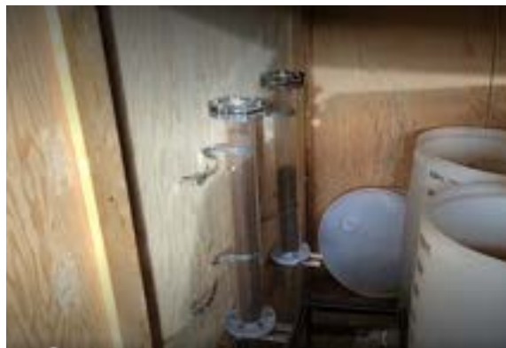
Figure 4: Columns C1 and C1b installed in series of BR1 and BR1b in the onsite research shed.
