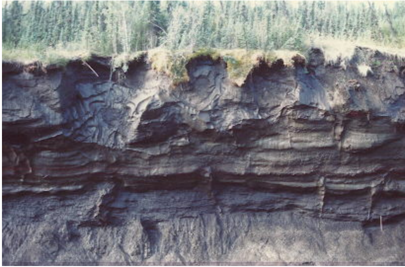
Figure 11: Ice-rich sediments, Last Chance Creek. These sediments are dominated by ice wedges in the upper half of the exposure, and segregated ice towards the bottom. Visually estimating the volume of ice wedges is essential in assessing the potential amount of sediment to be released upon thawing.
