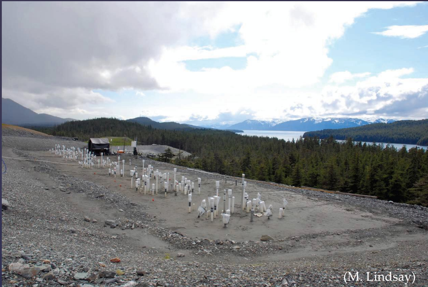
View of carbon amendment test cells and instrumentation on the Greens Creek tailings pile
