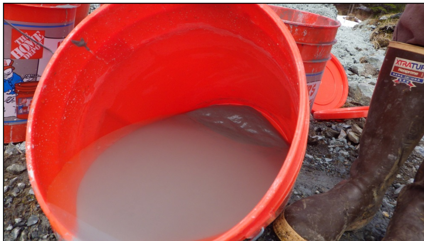
Figure 3.—Decanting supernatant water after tailings wash.
