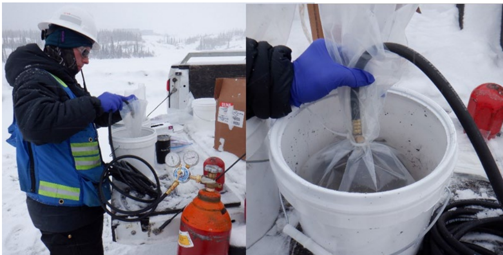
Figure 3-2: Tailings sample being purged with nitrogen gas before sealing sample bag in the field. Each bucket was then purged and sealed.
