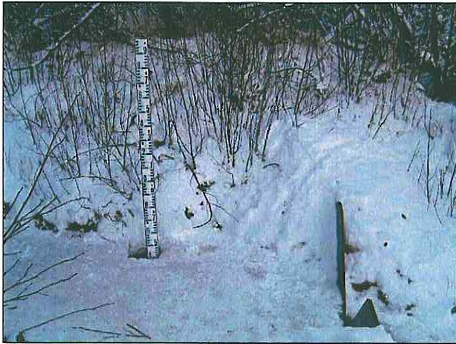
Plate 3 Staff Gauge Install (Water Level = 0.36m)
