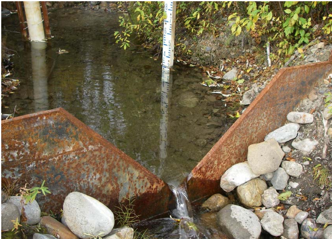
Photo C-4: V-notch weir and staff gauge on Grum Creek.
