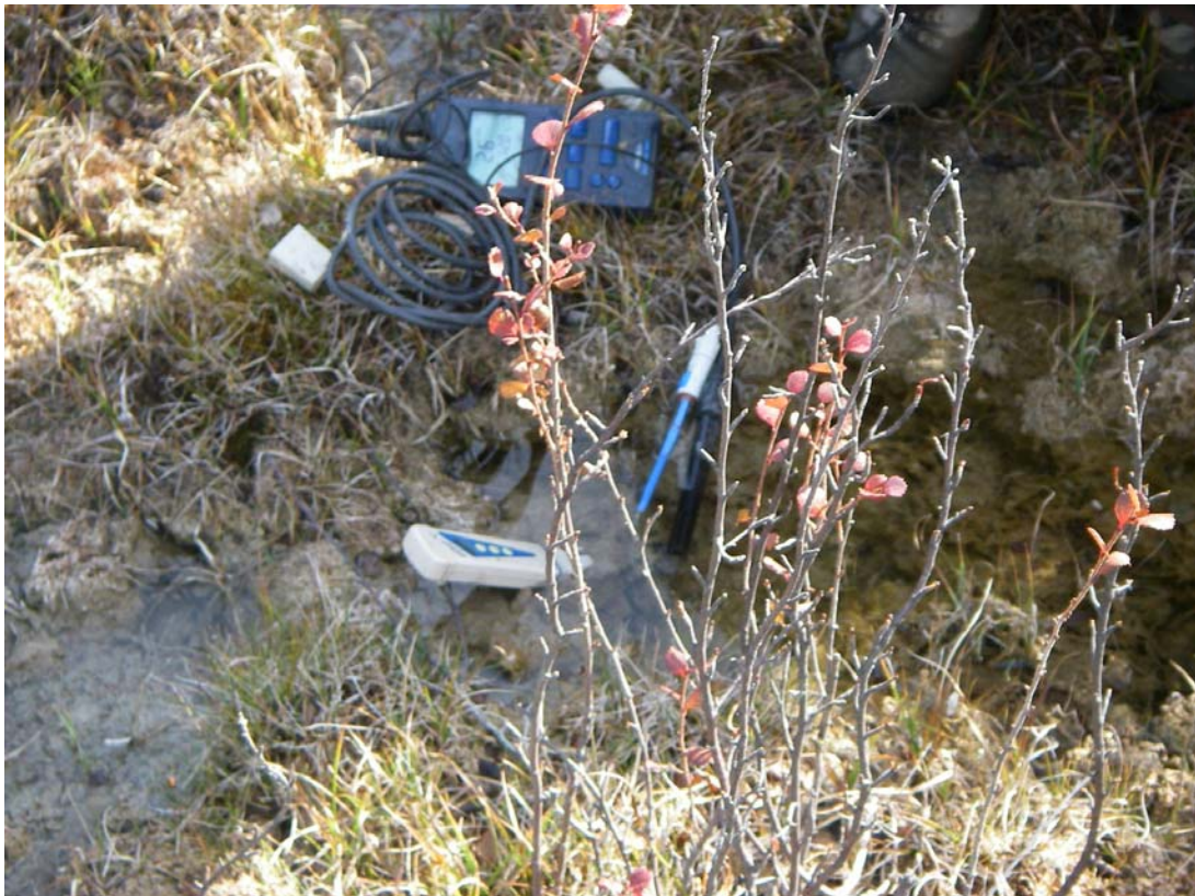
Photo C-2: Field pH, temperature, redox, conductivity and flow readings.
