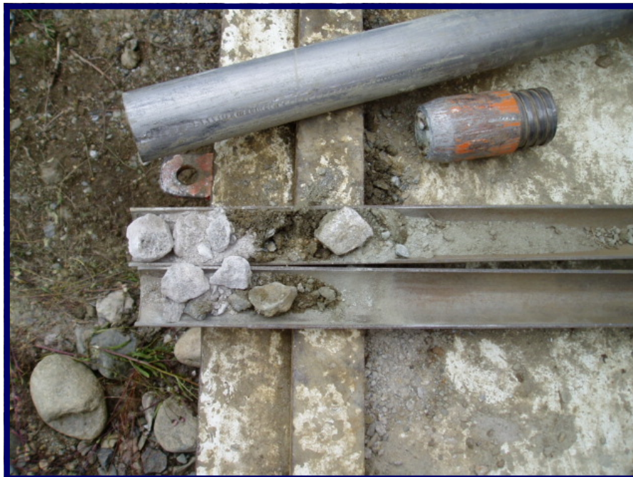
Photo 10 Close up view of sample JMS 21 retrieved from SPT spoon in BGC05-06 (9.75 m).
