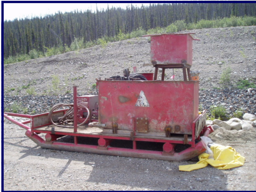
Photo 3 View of grout plant (on sled) used to mix grout for backfilling boreholes around instruments.
