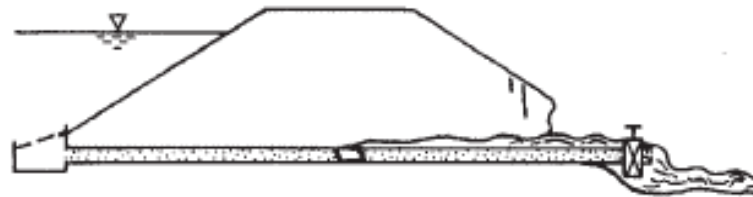
B - Hole enlarges allowing increased flow and a piping failure begins.
