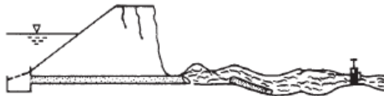
C - Reservoir drains through the conduit.
