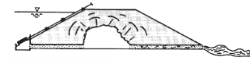
B - Hole in Conduit enlarges, cavity develops. Debris partially blocks outlet.
