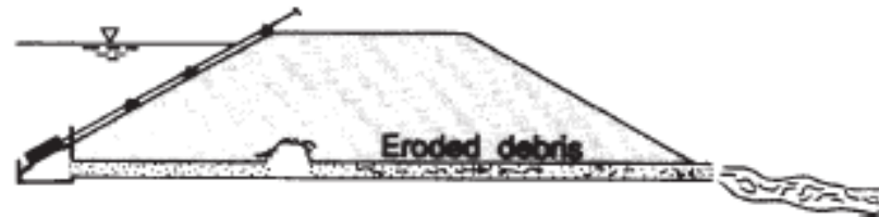
A - Hole develops in conduit, eroding embankment
