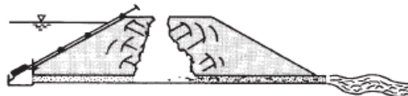
C - Sinkhole develops, complete failure is probable.
