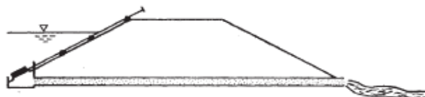
C - Inclined Slidegate
