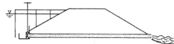
D - Vertical Slidegate & Catwalk
