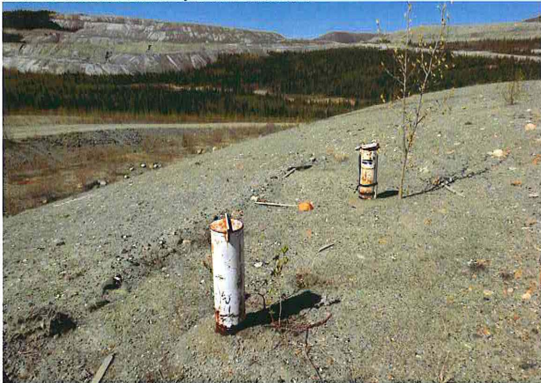
Photo 12: Piezometers 94-2A and 2B
