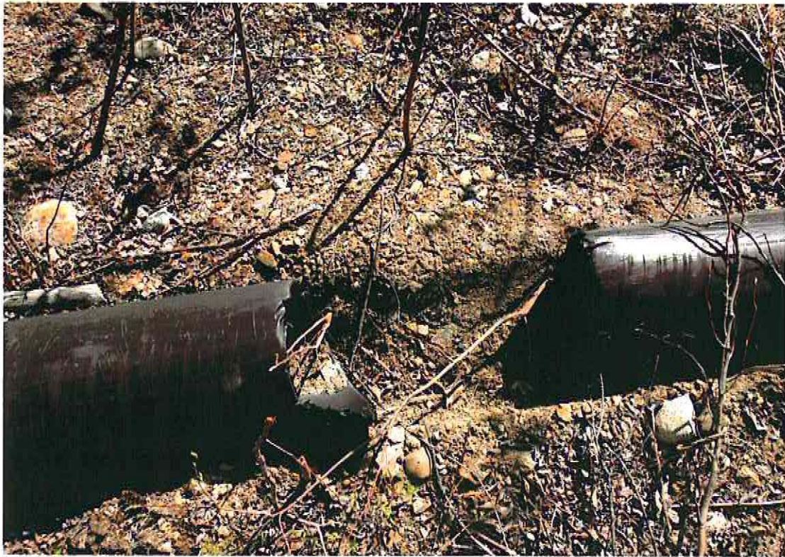
Photo 31: Break in siphon line from Moose Pond
