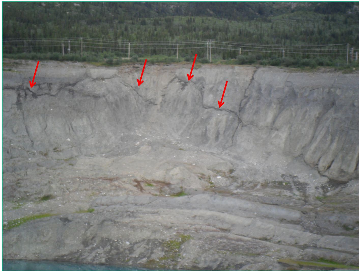
Photograph D-2 Grum Pit Instability Zone – new cracks reported in August 2012 indicated by red arrows. View looking east.
