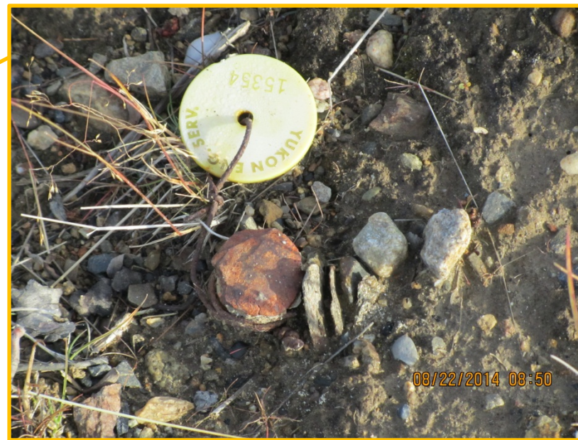
15342 PIN AND TAG IN GOOD CONDITION
