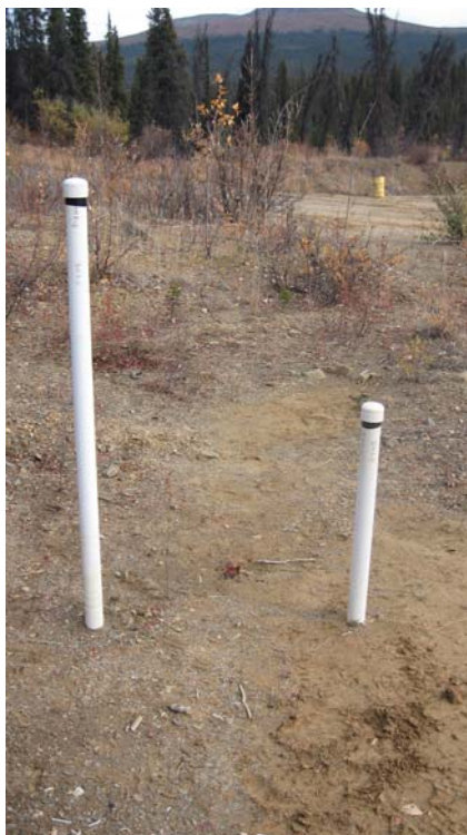
Photograph 9. Wells BH7S (tallest) and BH7D (shortest) – after investigation and BH7D pushed deeper
