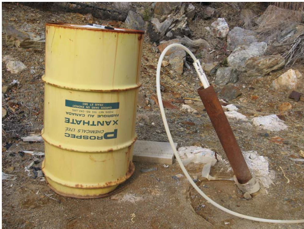
Photograph 6. Well BH10 A,B, well and steel casing are inclined at ground surface. (September, 2006)
