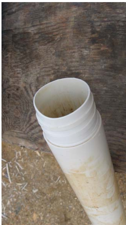
Photograph 5. Top section of well casing at BH7D after it was removed from ground and cleaned.
