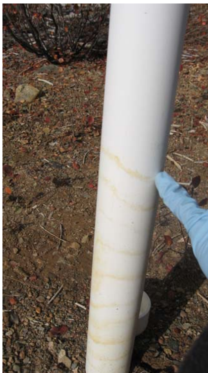
Photograph 3. Frost jacking lines at base of well BH7S
