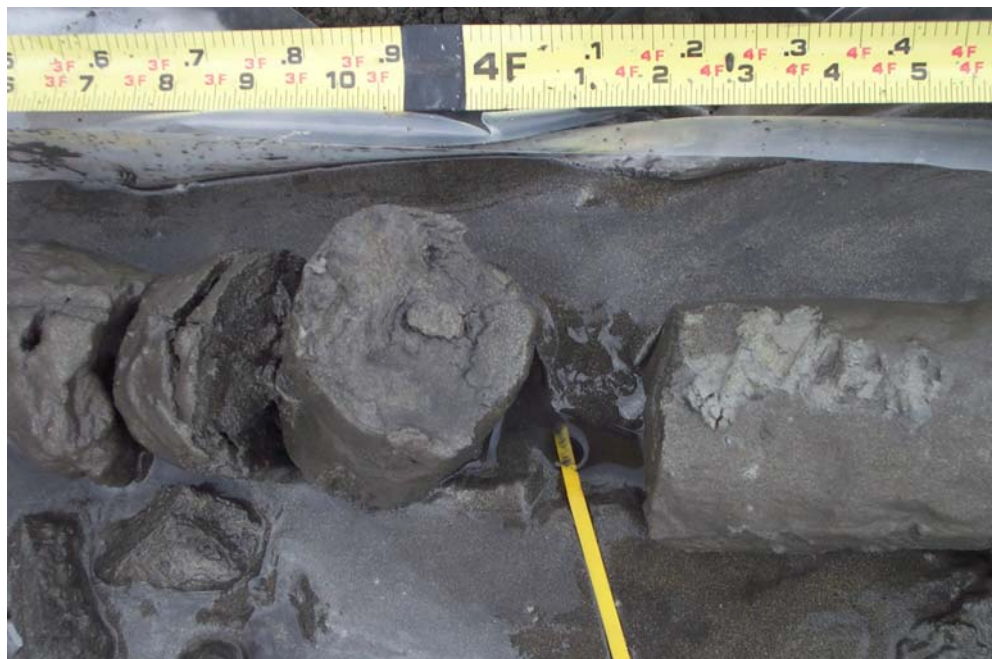
Photograph 2. Detailed view of frozen tailings (perma-frost) zone at depth of approximately 38.5 - 40 ft (11.7 – 12.2 m bgs) during installation (photo from Sept. 1, 2003)
