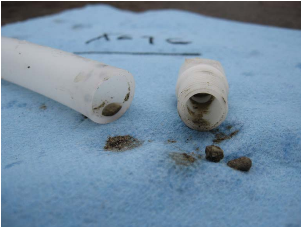
Photograph 4. X24C-96 – small rocks and sand clogging foot valve (August 2006)
