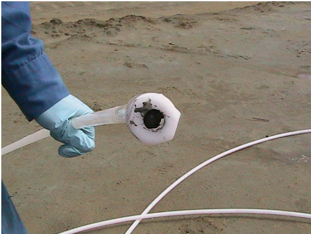
Photograph 4. Well X21C-96, foot valve clogged with what appears to be tailings tailings (July, 2005)
