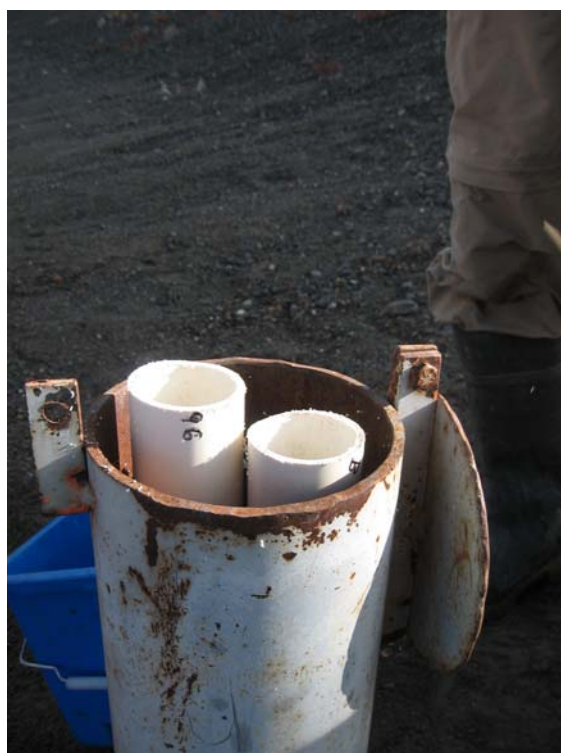
Photograph 2. Wells X25-96 after shortening stickup (Sept 21, 2006).
