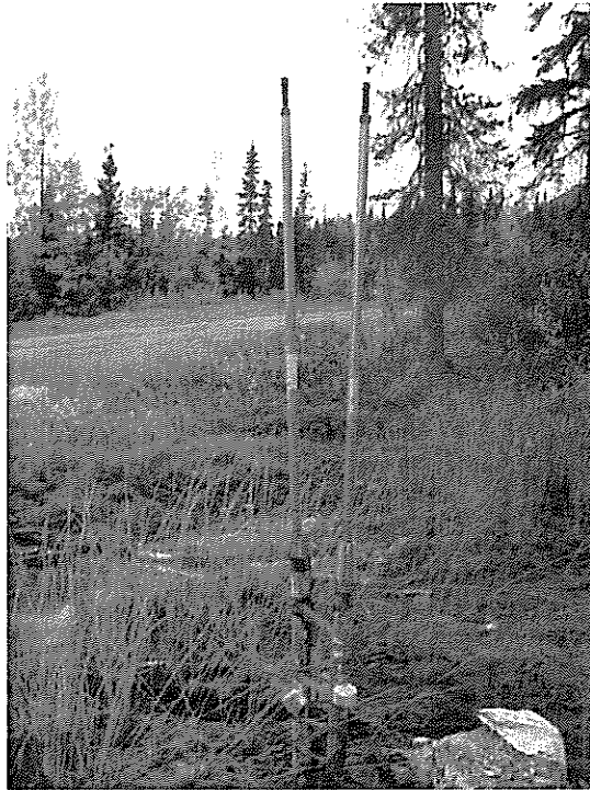
Photograph 7. Well SRK04-05 A,B. Nested artesian wells with mechanical packers. (Sept. 2006)
