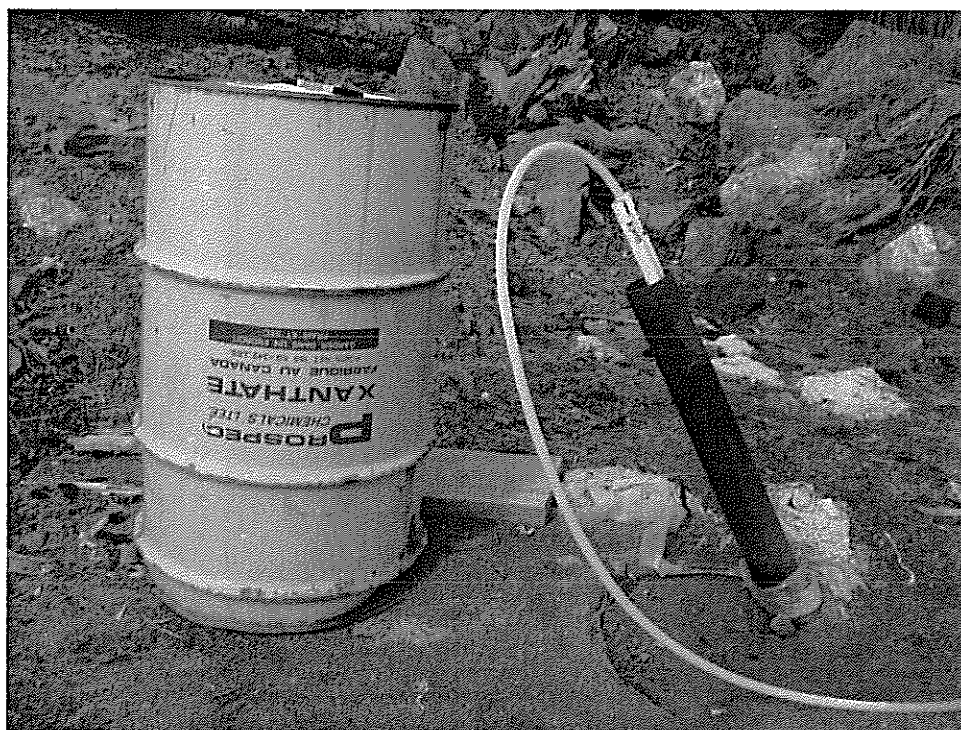
Photograph 6. Well BH10 A,B, well and steel casing are inclined at ground surface. (September, 2006)
