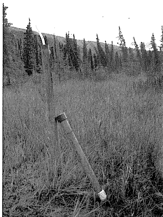
Photograph 9. Well S3 with top part of well casing extension removed. Top of well taken as top of section with tubing sticking out.
