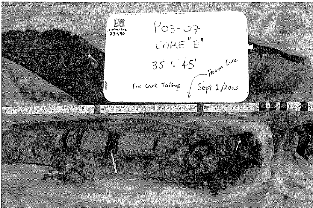
Photograph 1. Frozen tailings (perma-frost) zone at depth of approximately 38.5 - 40 ft (11.7 - 12.2 m bgs) during installation (photo from Sept. 1, 2003)
