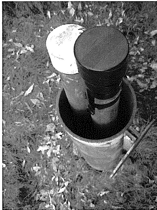
Photograph 3. Wells at P96-9 A/B. Well P96-9B was capped and taped shut because it is inoperable
