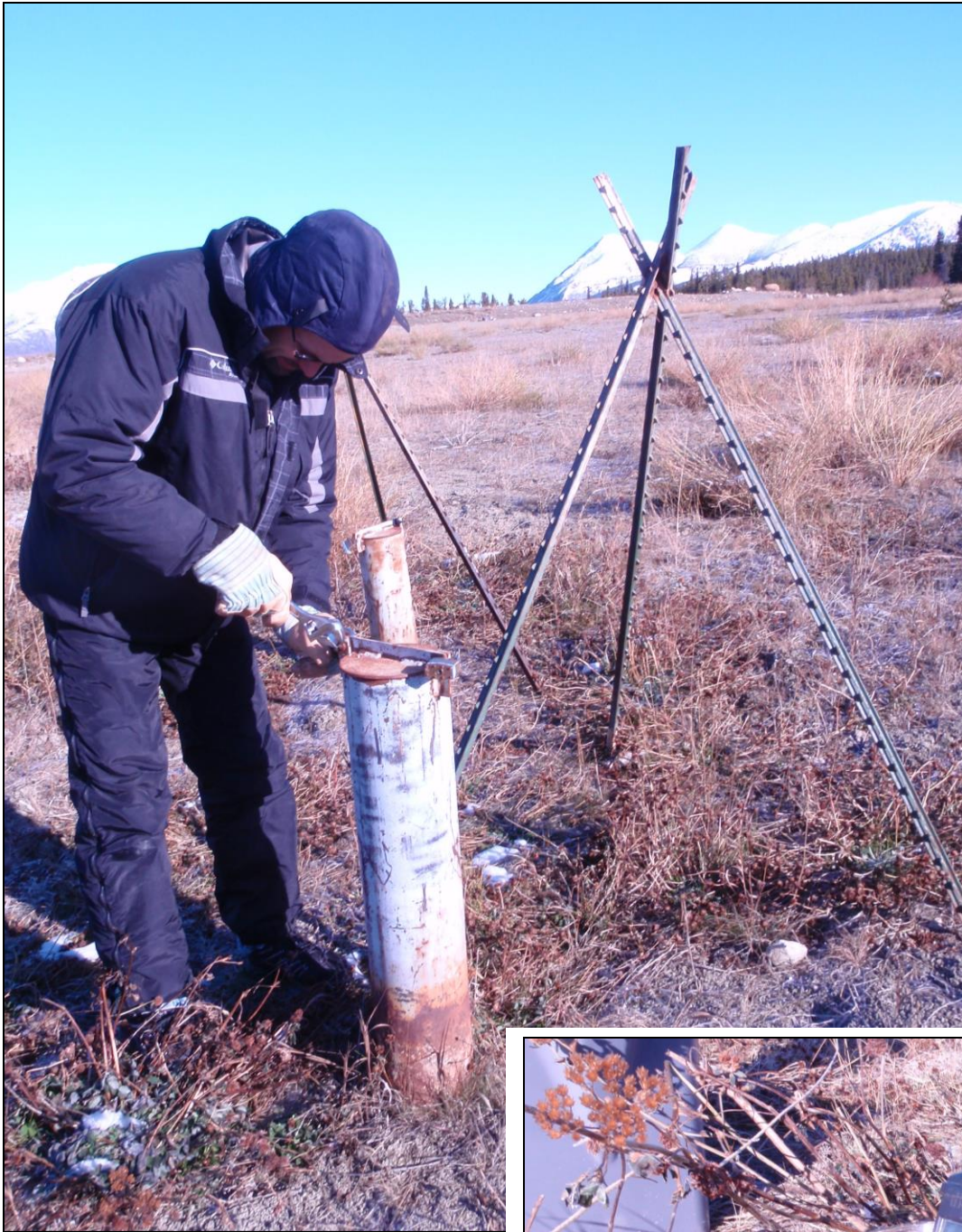
Photograph 4 & 3: Top-Waste Management Personnel removing the top from the monitoring well. Bottom- Multi-checker taking sample readings from (MW-1D) monitoring well
