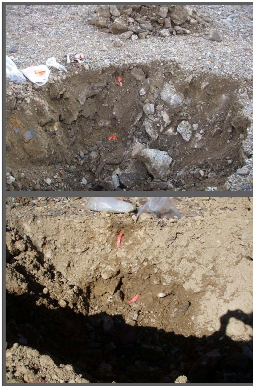
Photo 5e Example of physical and geochemical variability in the waste rock pile, test pit TP-9, South Pile, and TP-19, West Lower Pile. Both pits are 1 metre in depth.
