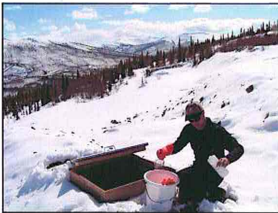
Plate 2 – ACG employee sampling at the Galkeno 300 treatment pond decant sampling box
