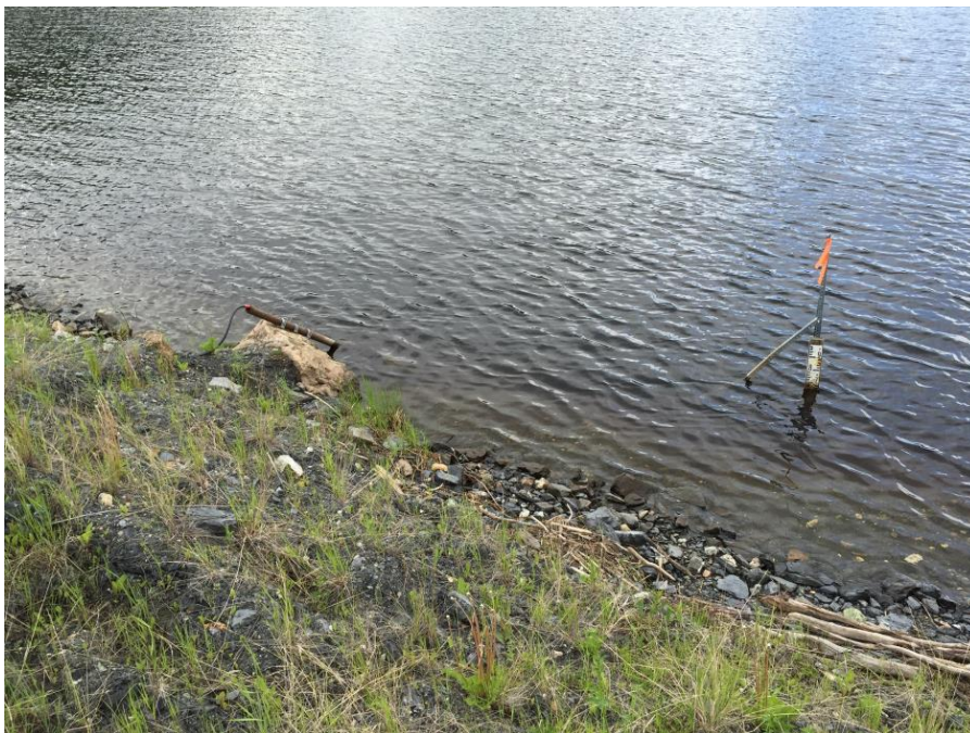
Photo 11 Level logger and staff gauge installed in Hugdeon Lake in 2015
