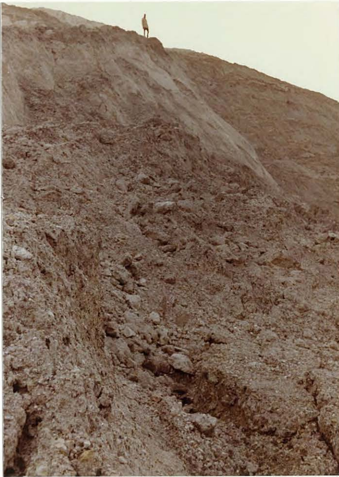
Photo 13: Uppermost section of the north lobe shows significant vertical displacement.
