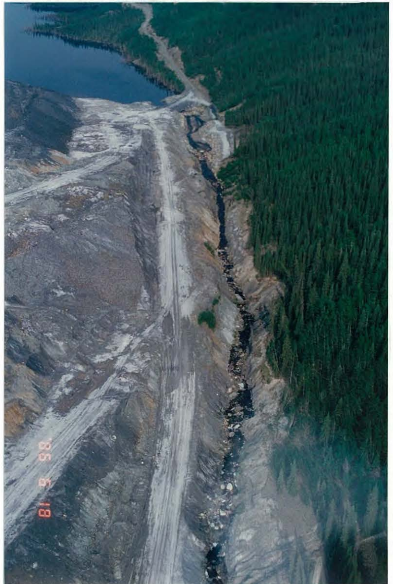
Photo 3: Fresh cracks in the headscarp of the waste dump confirm recent movements.
