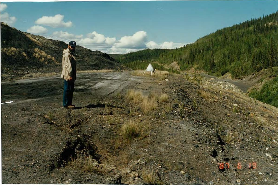
Photo 3: Tension cracks traverse the creek bank and access road. Sharp crack edges confirm recent movements.
