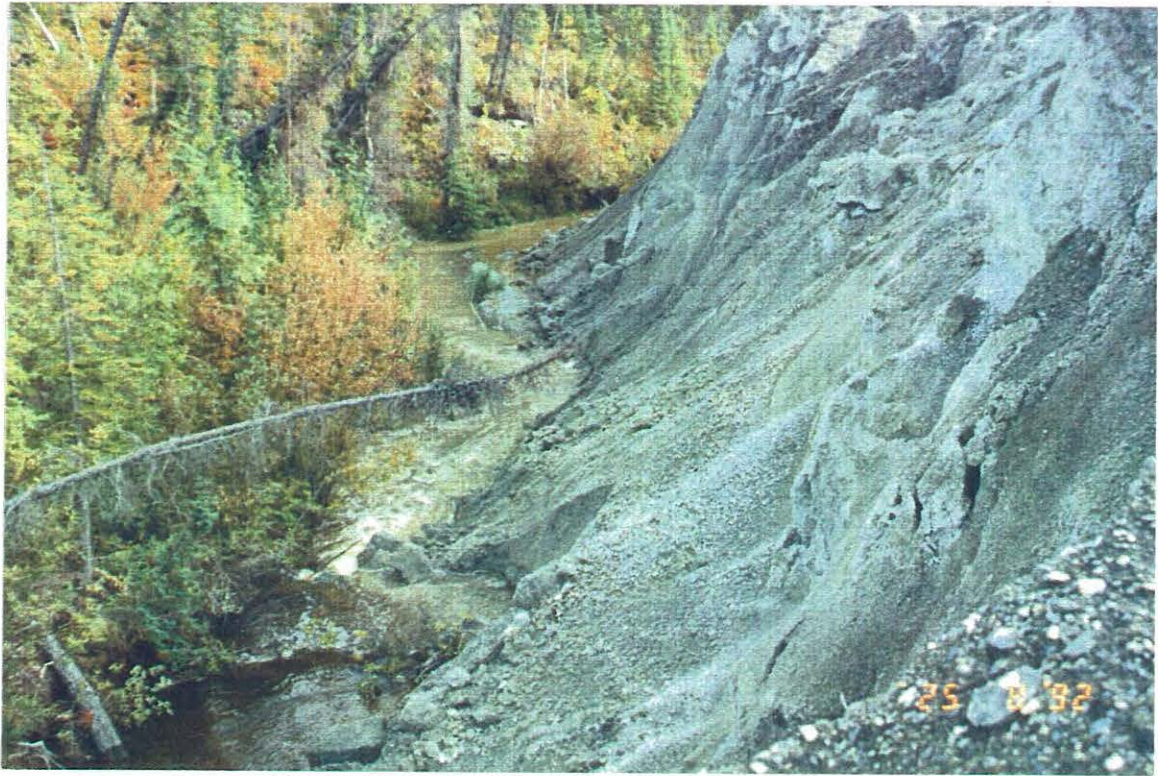
Photo 17: View of the upstream section of the south lobe impinging on the Clinton Creek channel. Note recent blockage being eroded.
