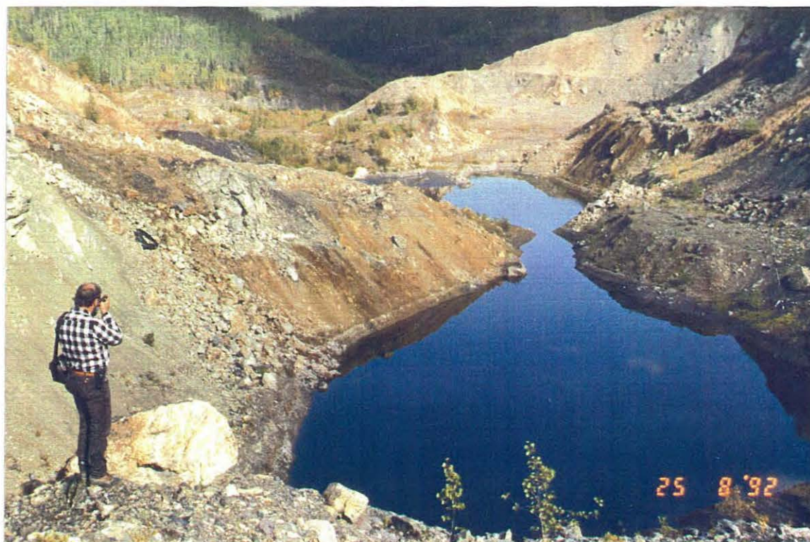
Photo 15: Seepage from the Porcupine Creek dump flows into a lake formed in the valley a short distance downstream.
