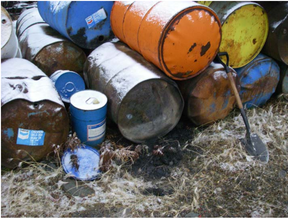
Photo #5: Surface stain near fuel storage area #1
