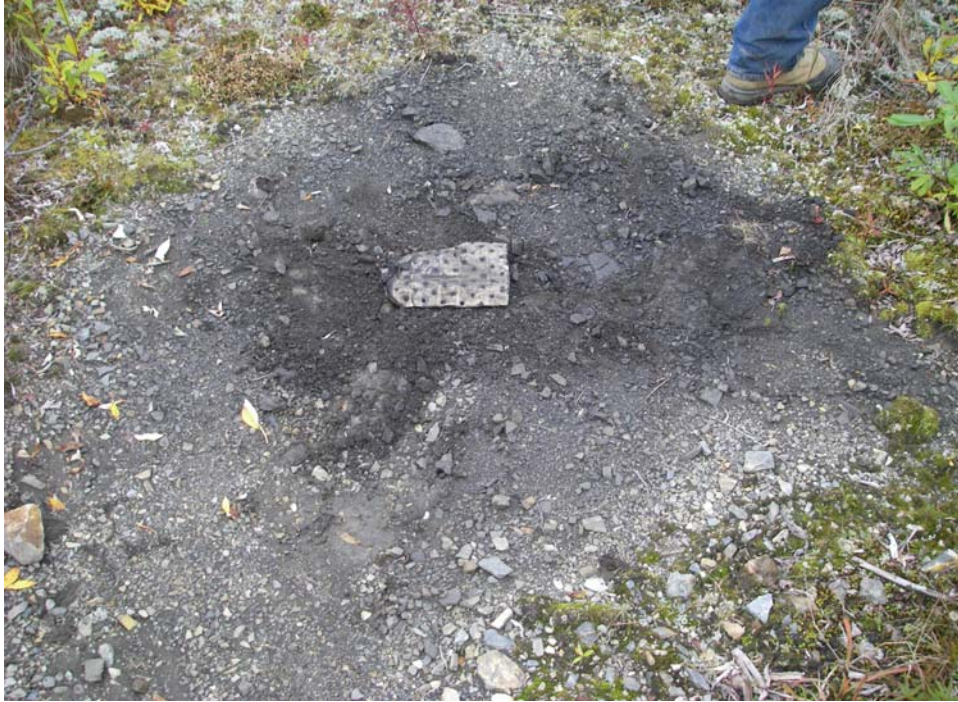
Photo #17: Surface staining with old oil filter near old dump at Bermingham pit
