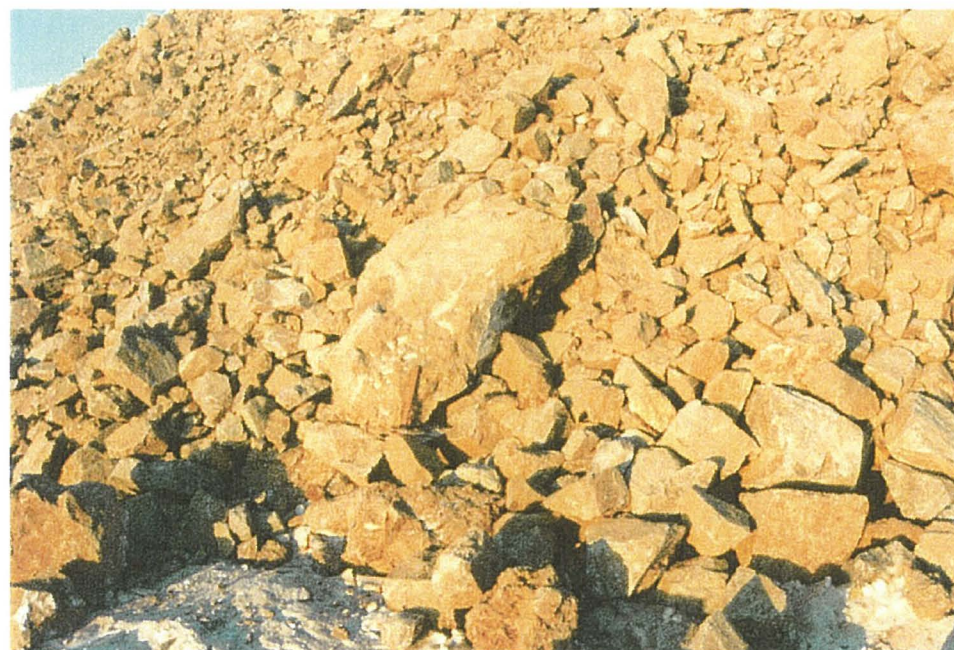
(February 14, 2001) Blasted riprap in quarry. Largest dimension (hammer) is 1.2 m.
