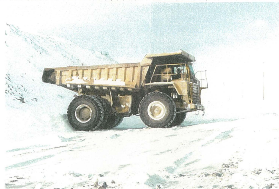
(February 13, 2001) Cat 773B rock truck used to haul riprap.
