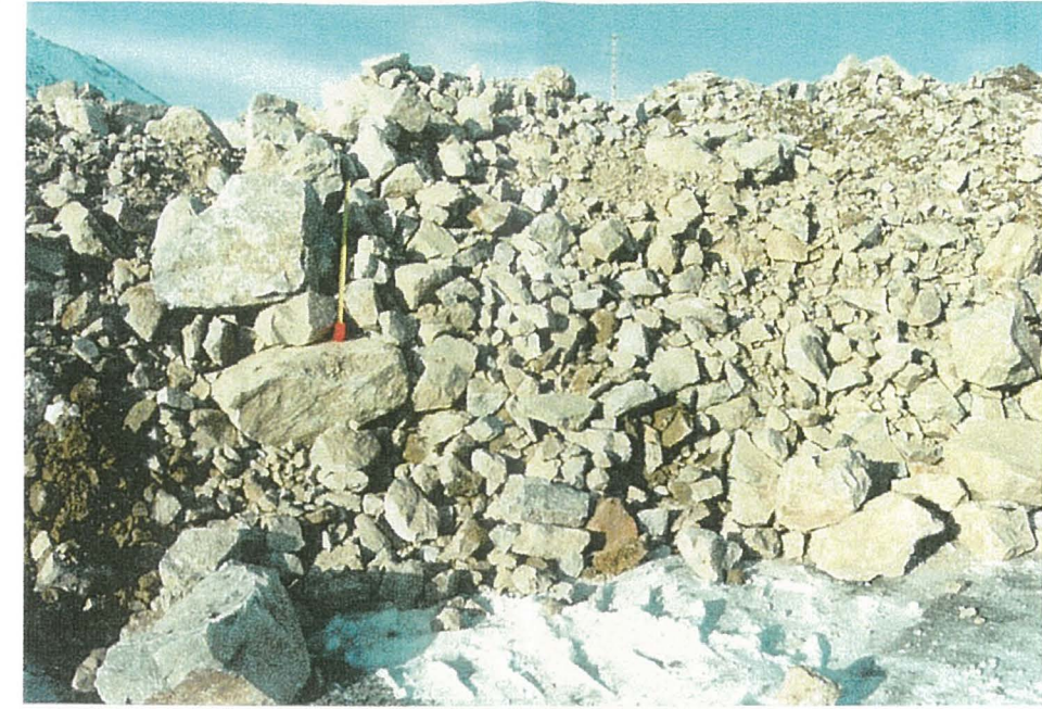
(February 15, 2001) Typical size, gradation of riprap in stockpile. Length of tape is 900 mm - maximum particle size specified.
