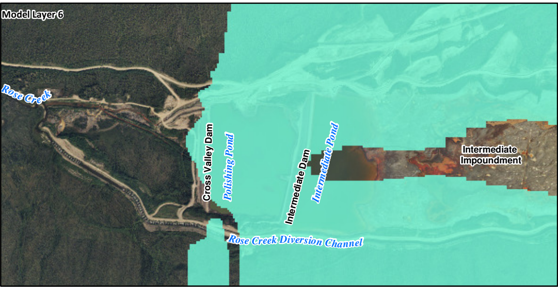
FIGURE 15 Modelled Hydraulic Capture Downgradient from the Cross Valley Dam Under Assumed Operation of SIS Scenario C1 Faro Mine Remediation Project
