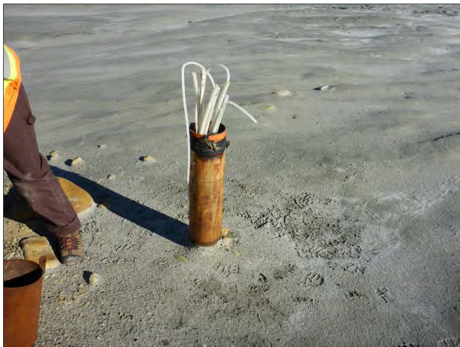
Photo 25: View of well P03-06, includes depths 1, 2, 03, 04, and 05. Photo taken on September 21 st , 2016.
