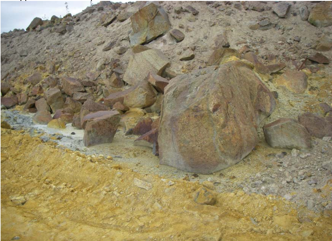
Photo 10: Regions of high sulphide content waste (whitish-grey) remaining at from the fringes of S/P2.
