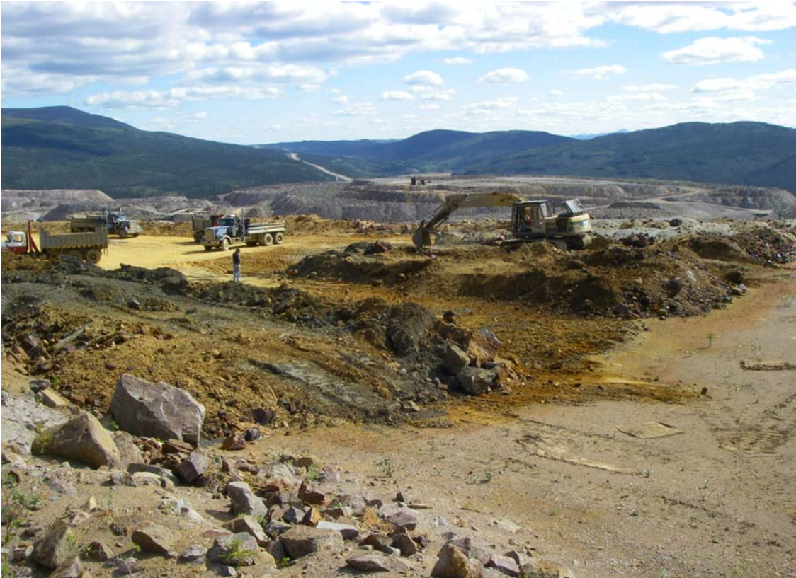
Photo 7: The waste from S/P2 was loaded selectively to segregate the wet fines (grey colour) and the dry material (orange).
