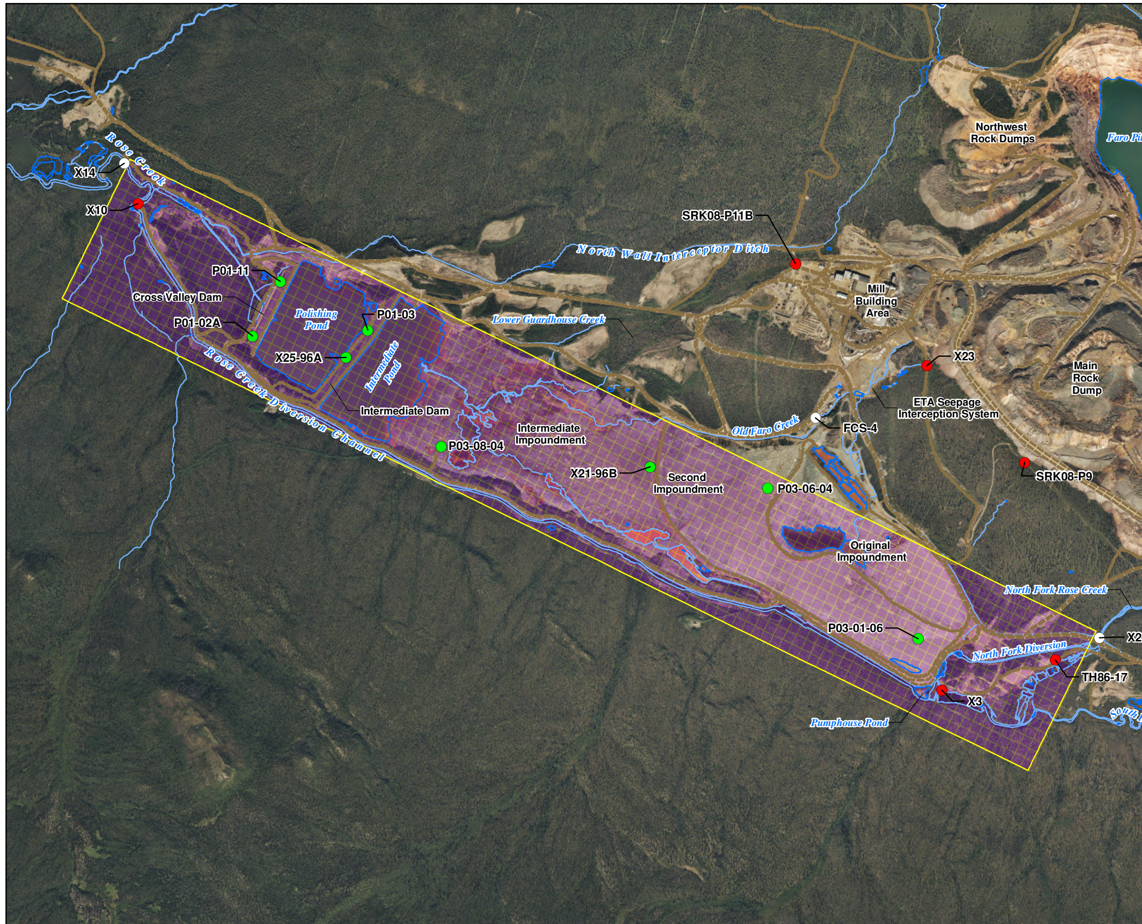
FIGURE 4-9 PHAST Model Grid Faro Mine Remediation Project
