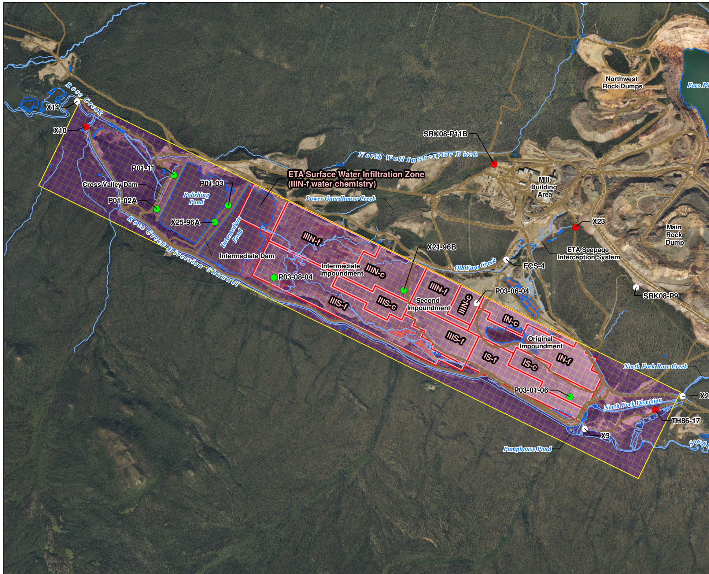
FIGURE 4-12 PHAST Model Infiltration Boundary Zones Faro Mine Remediation Project
