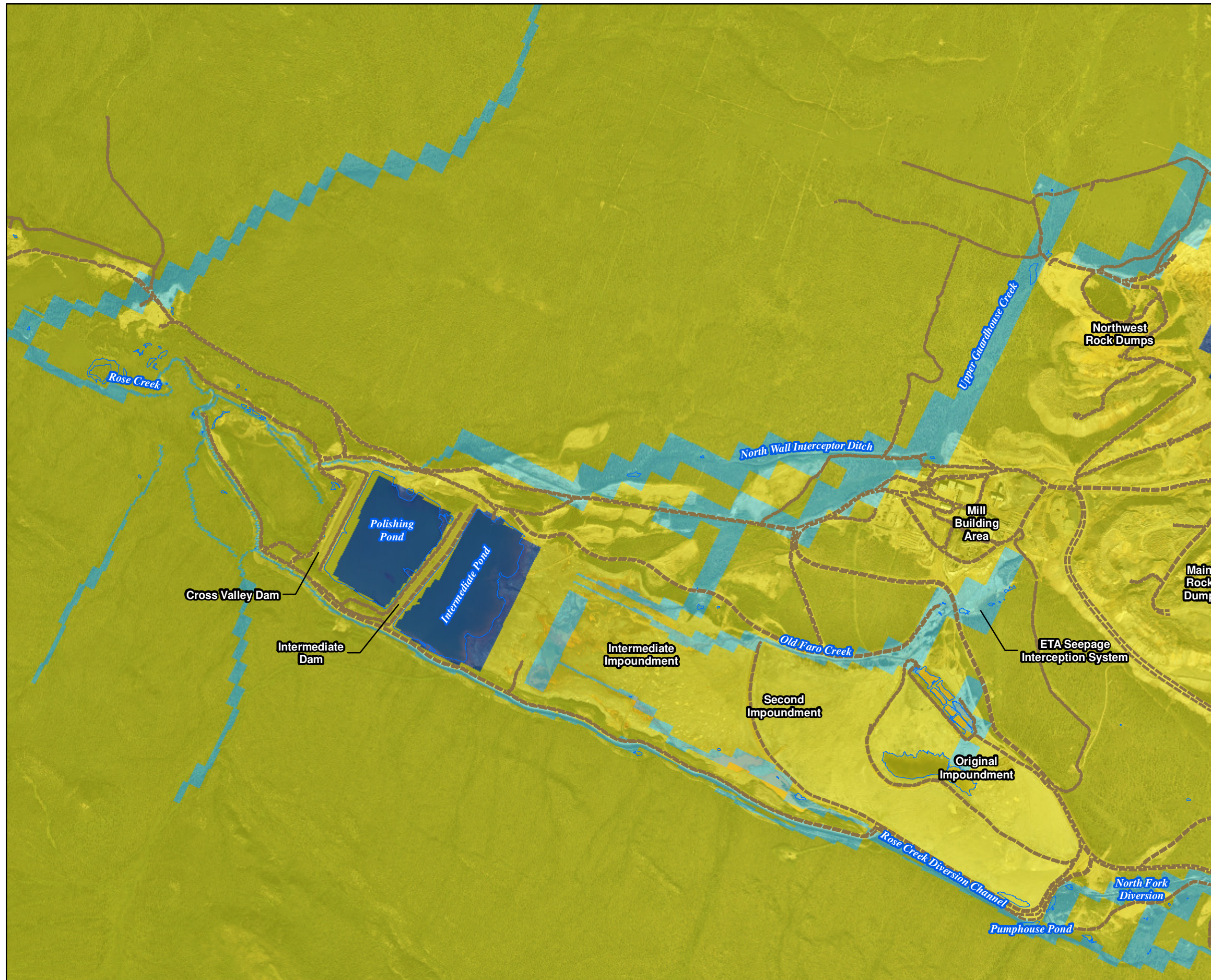
FIGURE 3-12 Groundwater Flow Model Boundary Conditions: RCAA Subarea Model Faro Mine Remediation Project
