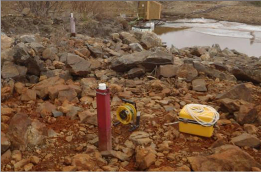
Photo 13: MW09-21, West and Upgradient of Seepage Pond. Note seepage pond and pumphouse in background and levellogger cable wrapped around the top of the protective casing. June 3, 2012
