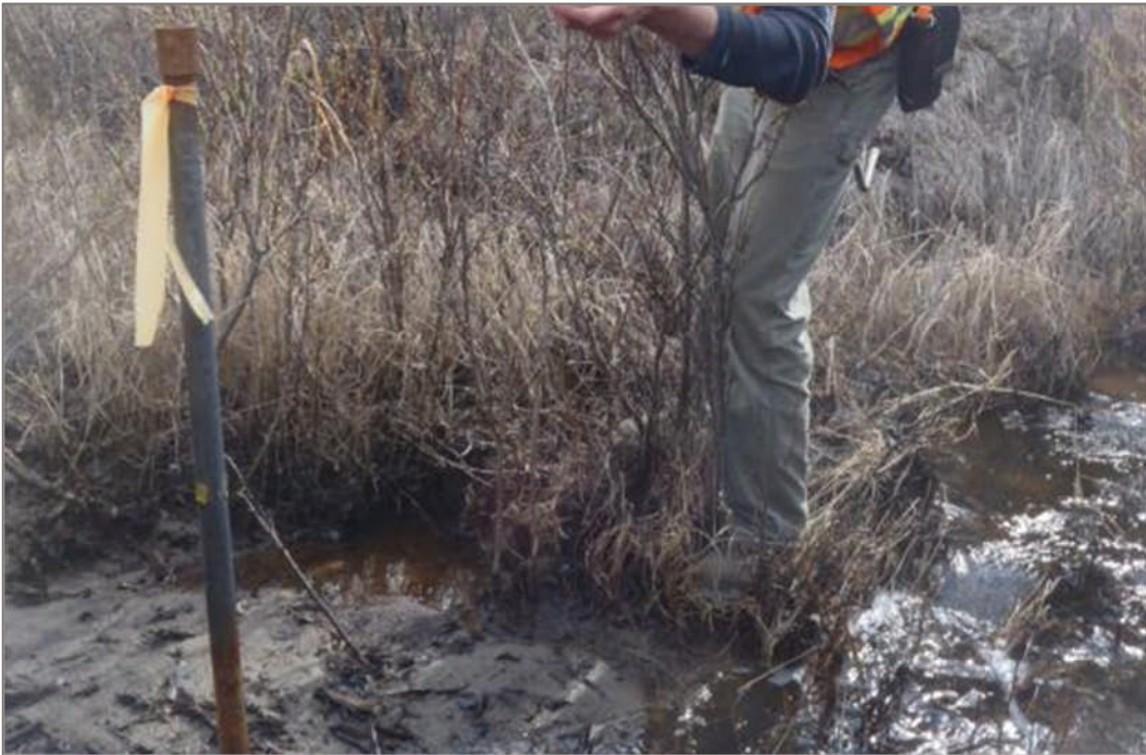
Photo 18: MP09-02 Drive-Point Well in Pony Creek. June 4, 2012
