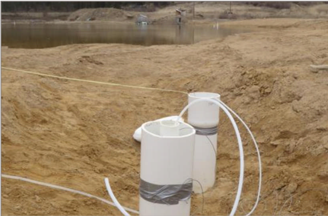
Photo 2: MW09-03 and MW09-04 in the Southeast Tailings. Note the cable in each well used to suspend Solinst Leveloggers. June 2, 2012
