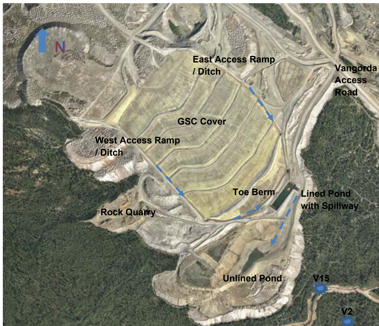
Photo 2-1. Aerial view of Grum Dump with GSC Cover, perimeter ditches, ponds and select monitoring stations at the toe.
