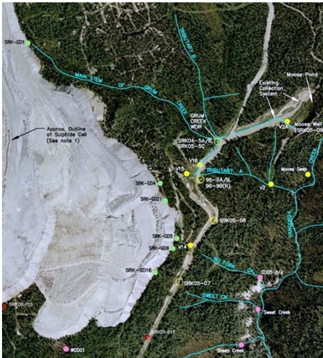
Photo 4-1. Aerial view of water quality and seepage stations located at toe of Grum Dump (after SRK February 2011).
